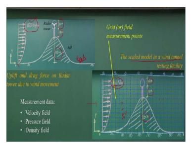
That they let be there is a weather radar is there. You know it nowadays weather radars are there to measure the rainfall, the wind velocities and all. That is what is a on the hilltop and it has a stand of 10 meters and the weather radar tower is about 10 meters. And the wind is moving at a speed of 150 km/hr and the velocity is 0 at this point.
