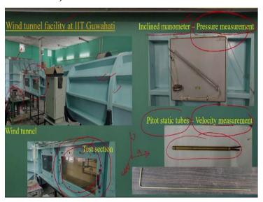
For example, if you look it that point, like the wind tunnel facilities what you have at the IIT Guwahati in the Department of Mechanical Energy. See if you can look at this wind tunnel the setups okay there is an inflow, this will be the outflow and this is what the test sections what is there and these are all the recording systems for velocity measurement and the pressure measurements.
