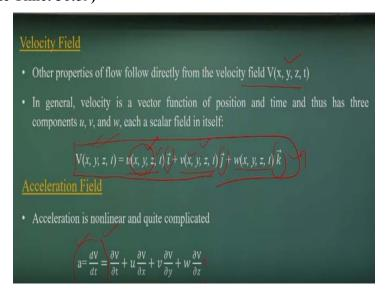
So now I am just defining them the velocity field, when we are talking about we are talking this velocity as a vector quantity, which vary in a space in case of the Cartesian coordinate system of x, y, z and the time. But most often for easy point of view, we resolve this velocity vector component into its scalar component in Cartesian coordinate systems like the i and j and k.
