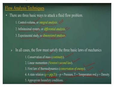
Now if you let me summarize that way, there are three basic ways to solve the problems. One is a bigger control volume where we have an integral analysis or the analytical methods ways. You take a smaller control volume, which is very close to infinitely small. Then you get a set of a differential equation problem. So that is the reason we call differential analysis.
