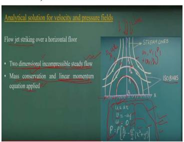
Second one you know it we are looking for a analytical solutions. That means the fluid flow problems we are more or less very simplified cases like for examples, we have a flow jet, that means flow velocity is coming from this striking on the horizontal floor here. The flow jet is coming and striking over a horizontal floor. And our interest to know it what will be the pressure distributions, what will be the velocity distributions.
