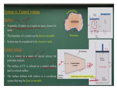
First let us talk what is the system, what is the control volume. The system is a quantity of matter or the region in a space chosen for the study. For example, I have considered a 2 kg of gas which is having 1 meter cube volumes. And if I heat this gas, if I give a temperature to this gas, then what will happen? This gas will be expanded.
