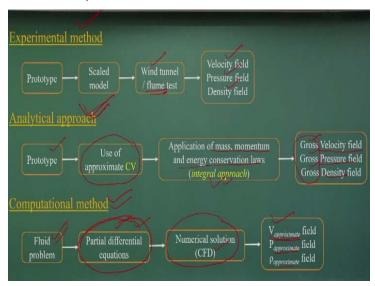
So similar way, that is what I am telling it, there are three ways to do the solve the any flow complex flow problems, like you can have experimental methods. That means you can have a prototype and make a scaled models. That means you can reduce the flow and the geometry of the problem in such a way that you do a scaled model.
