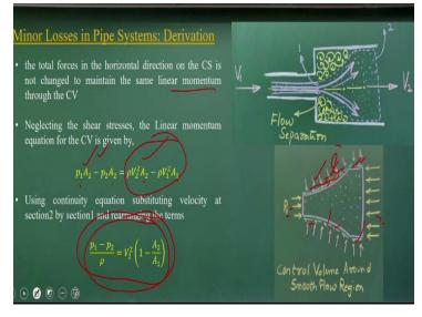
Now coming to this, I am just applying the linear momentum equations for these control volumes okay. So if you have this is the control volumes. So you may have the shear stress is acting on this okay, this the shear stress part, okay. But we are neglecting this part, we are neglecting the shear stress part. Just we are assuming the pressure different between these is equate with a momentum flux.
