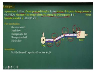
So now let us come to the questions okay, the examples what we have. Okay, so the first example is very simple is there is a pump okay and which moves this amount of the waters per second. That means, this is given to us, through a pipe diameter is given is a pump discharge pressure is this much okay kilo Pascals. What must be the pressure of the flow entering the device at the position B, okay.
