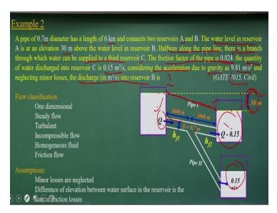
Now you take it the second problems which has the GATE 2015 problems is that the pipe of 0.7 meter diameter has a length of 6 kilometer connects the two reservoirs okay and the water level in the reservoirs is 30 meter above the water level of reservoir B okay. Halfway along this pipeline there is a branch. Water is supplied to the third reservoir C. Then friction factors of the pipe is given.
