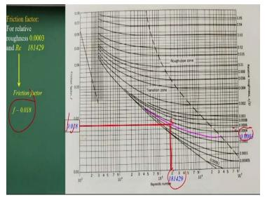
Identify this approximately which the curve will come there. You know, these Reynolds number, compute it that. Draw the lines with matching that then compute this friction factors, okay? It is very easy. Using this Moody's diagrams, you can first identify with respect to the relative which curve we should follow it. But if curve is not there exactly we can interpolate it that curve and know the Reynolds numbers, interpolate it this.
