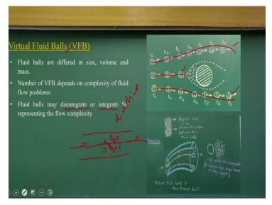
Now let us go for the next slides which is again I will talk about virtual fluid balls. Here again I have to repeat it to tell it the virtual fluid balls to understand how the vortex formations happens within a pipe flow systems, okay. Like the last class I discussed about the pipe flow systems, when I am considering it, the pipe, a horizontal pipes and because of the turbulence how the eddies formations happen.
