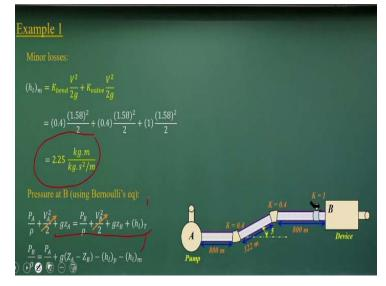
If are considering that the loss components will get it this much is the minor losses. Now we are substituting Bernoulli's equations, the modified Bernoulli's equations to compute what could be the pressure. So I am not going more detail as you can read this ppt to get these details.
