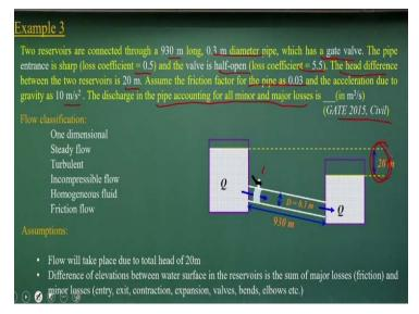
Another the third examples. Okay, two reservoirs are connected with a 930 meters. That is the GATE, again this 2015 paper. The diameter pipe which has a gate valve, okay it is having the valve here, okay. The pipe entrance is sharp. The loss coefficient is given it. The valve is half open. Loss coefficient also is given there. K is given here. Here also K is given. The head difference between two reservoirs is given it.
