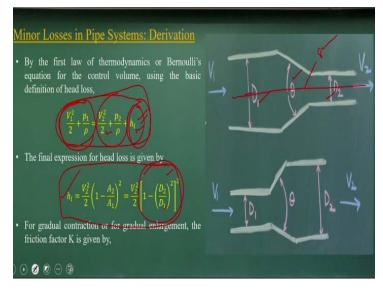
Now I will applying Bernoulli's equations along the straight line, okay I am just applying the Bernoulli's equation along the straight line. When you apply the Bernoulli's equations, this line is horizontal. This streamline is horizontal, so you do not have a z components. You have pressure head component and the velocity head component. That is what you equate,
