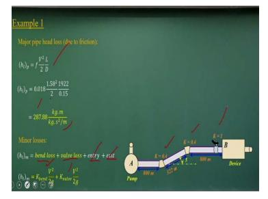
So that means I know the head losses that is what is computed here by substituting this value. There will be minor losses like bend losses, valve losses, the entry and exit losses all the components, this entry and exit loss we do not consider it here only the bend loss and valve loss we compute it which we have these values.
