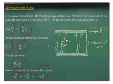
If I consider the same fluid flow through a parallel plate, okay. One of the plate the velocity is zero which is at the rest conditions and other the top plate is moving with a velocity V. So as a microscopic point of view I am not talking about the molecular motions or exchange of the molecular motions or the momentum flux that what is resulting a shear stress. Here what we consider that fluid element.
