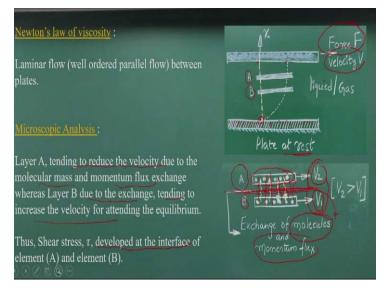
Now let us go to the very interesting concept, the Newton's laws of viscosities, okay, which is very simplified, simple common laws of viscosity which we use for solving many of the problems in laminar and also approximate for other flow conditions. Let us talk about this Newton's laws of viscosity. I am presenting you in two ways. One is microscopic analysis and the macroscopic analysis.
