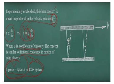
And shear stress will develop at this interfaces level and many of the studies the experimentally establish that this shear stress will have a directly proportional to the velocity gradient okay. If the more the they have the directly proportionality okay. That means more the velocity gradients is there so we will have the more shear stress. But it has a directly proportionality quantity.
