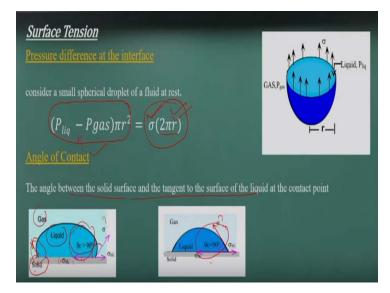
If you have the surface tension if you can now there will be a net balancing effect of the force component which results us the pressure difference. Let us consider it is the surface tension is given very simple examples of raindrops okay. Any raindrop if you look at that, if you take that drop and make it two splits. At the interface surface there will be surface tension is working it.
