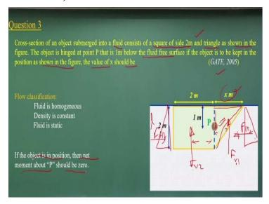
Now let us come to the another questions number 3, the cross sections of object submerged into a fluid consists of a square side of 2 meters and the triangle as shown in the figure. Object is hinged at the point P is 1 meter below the fluid free surface if object is to be kept in this position as shown in the figure, the value of x should be what is the x value so that this will be at a same position, the equilibrium positions.
