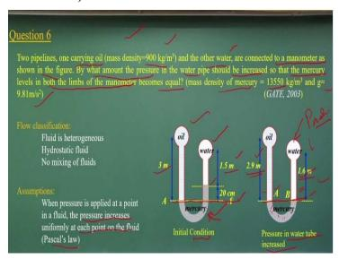
The question number 6, that is what two pipelines one carrying oil. The mass density of the oil is 900 kg per meter cube. Other one is water. It is connected to a manometer as shown in the figures. By what amount of pressure in the water pipe should be increased so that the mercury levels in the both limbs of the manometers becomes equal.
