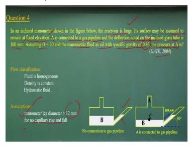
Now let us come it to a manometer problems. So there is a inclined manometer shown in the figure below. Reservoir is large. That is the, its surface maybe assumed to be remain as a fixed elevations. A is connected to a gas pipeline. The deflection is noted on the inclined gas tube. This is what the inclined gas tube is 100 millimeters the theta the angle of inclined manometers theta equal to 30 degrees and manometric fluid as oil with a specific gravity of 0.86.
