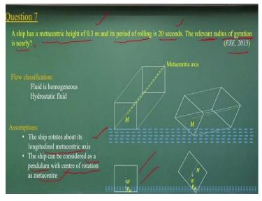
Now take it the question number 7. There is a ship of metacentric height of 0.3 meters. Its period of rolling is 20 seconds. The relevant radius of gyrations is nearly or what is
