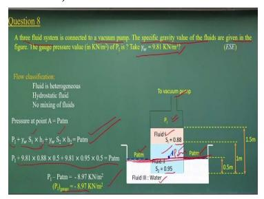
Now take it the question number 8, which is a three fluid system connected to a vacuum pump okay, where there is no pressures on this. So that is what the vacuum pump. Specific gravity values are given in these figures. Okay that is a S 1 is 0.88, 0.95 and the water which is specific gravity equal to 1. Then this gauge pressure value at P 1 what will be the pressure at the P 1 value if you consider the unit weight of the waters 9.81 kilometer per meter cube.
