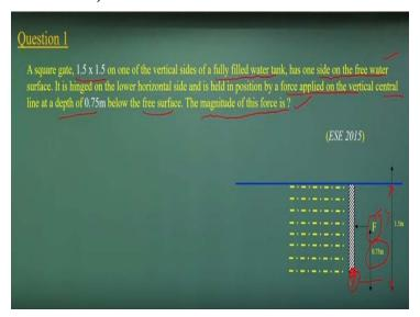
Let us start to solve the problems, these very easy problems that there is a square gate of a dimensions of 1.5 meter into 1.5 meters. One of the vertical sides of a fully filled water tank has one side on the free surface. It is hinged on the lower horizontal sides. Here it is a hinged it and is held in a positions by force applied on the vertical the central line at a depth of 0.75 meter below the free surface.
