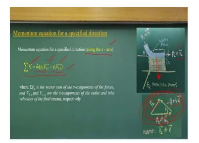
Now, there are the problems where is come it, very interestingly that we can apply the momentum equations as you can go it, this momentum equation is a vector equation, it has a three components in scalar directions, X component, Y component, Z component. Many of the time, we result at specific directions, in this case is X directions to find out the force components. That is what we try to look it, what will be the force is happening it, in the X directions only.
