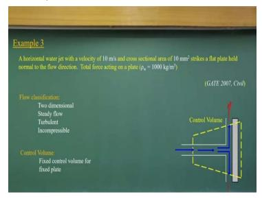
[A horizontal water jet with a velocity of 10 m/s and cross sectional area of 10 mm<sup>2</sup> strikes a flat plate held normal to the flow direction. Total force acting on a plate ( $\rho_w = 1000 \text{ kg/m}^3$ )] Flow classification:
