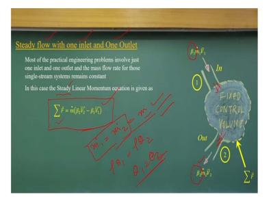
Now, let us go for another simplifications. That in a steady flow conditions, okay and only one outlet one inlet, this is very simplified case. See when you have one inlet and one outlet, if your mass influx is  $\dot{m}_1$  is inflow is coming into that, your mass influx out will be  $\dot{m}_2$ , that should be equal. That means,  $\rho Q_1 = \rho Q_2$  will be equal that means Q1 = Q2, that is a very basic equations what we get it, if we apply the conservations of mass.
