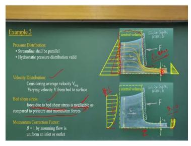
Now, first is pressure distribution. Now, if this is my control volume, first I need to draw the streamlines. So, as it expected that the streamlines will be like this, so as actual fluid valve if you have it could be like this, if the follow of actual fluid valve, if I follow it, it could be like this. So, we should consider the control volume such a way that, at a slow par distance such a way that all the streamlines should be the parallel, okay.
