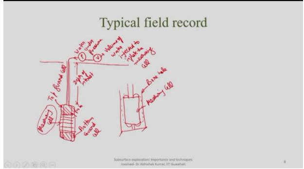
so there will be in addition to like we'll ensure like because you are interested to find out the deformation directly by correlating with the volume, so you ensure that the height in which the inflation is happening it's not changing, only inflation is happening in radial direction, so you only assume like inflation in radial direction, so whatever like the measuring cell which was before the start of the test was in cylindrical position, radial direction.
