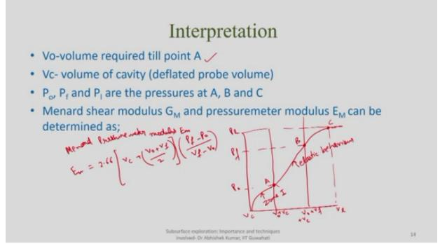
this alpha depends upon the soil type, charts are there based on which you can actually determine how much is the value of alpha. And then same way you can determine the value of un-drained shear strength that will be called as CU, that will be PL divided by 9 only for clays.
