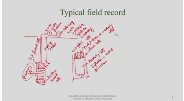
since the pressure is same in guarding cell, guard cell as well as in the measuring cell there will not be any end effect so whatever movement will be there that will be possible only in radial direction.
