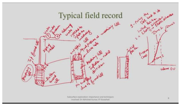
now you started pushing the soil, so by that time soil goes to its original position there will be too much change in the volume, but even for small pressures what you can see here after it reaches to its original position there will be actually loading of virgin soil kind of thing, so there will be linear pressure deformation characteristics which can be directly related to the volume also, because that deformation is happening in radial direction alone.
