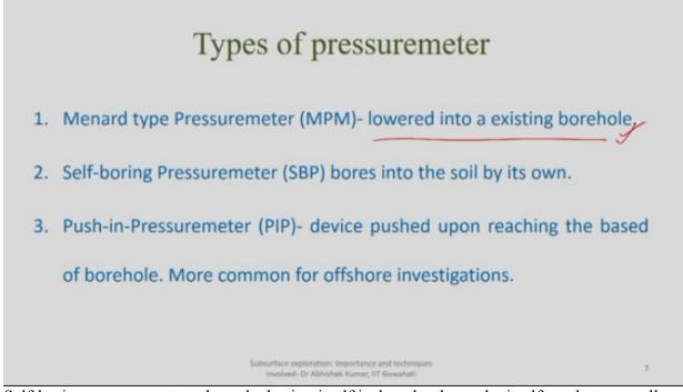
Self-boring pressuremeter where the boring itself is done by the probe itself, so that you call as self-boring pressuremeter or SBP.
