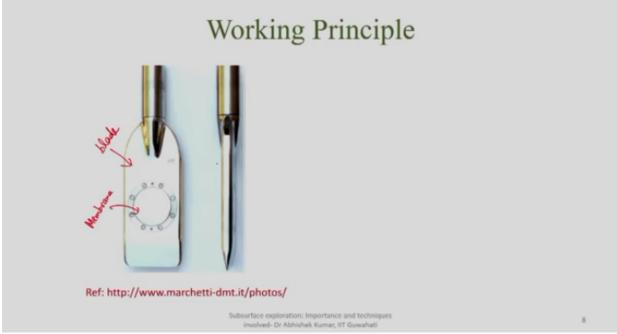
but in order to ensure or in order, so now we will be discussing how this membrane works, so if you take the cross section of this blade, so you will actually see some kind of arrangement like this, so there will be a spring which is connected to some assembly here, and this assemblies again connected here and there will be additional assembly, I'm going to nomenclature each of this assemblies here whatever I'm drawing for better understanding.
