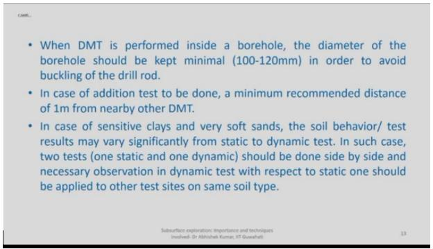
Again when the DMT is performed inside a borehole that diameter of the borehole should be kept minimal in order to avoid any kind of buckling to the drill rod.
