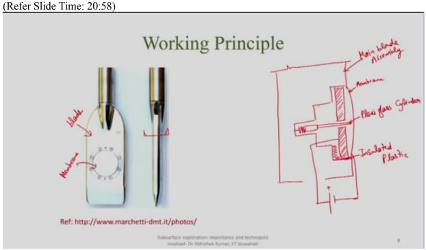
as we have been discussing like the movement of the blade will be detected by the spring this is called as again stainless steel cylinder. (Refer Slide Time: 21:14)
