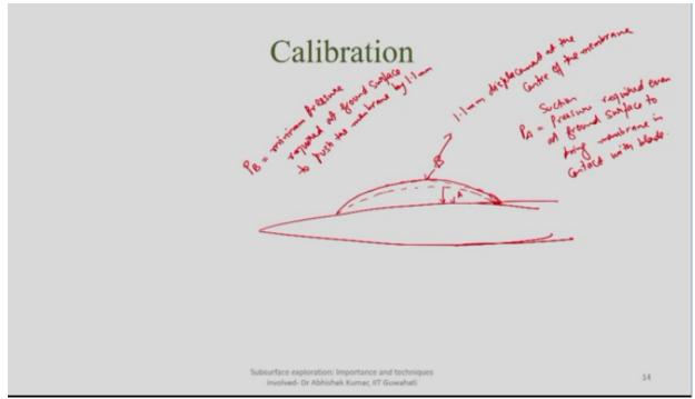
remember we were interested to find out the pressure required to push the soil by 1.1mm, but actually because of the membrane material some pressure will be required to bring, to push the membrane itself even when there is no soil, so this is some kind of additional calibration you have to do at the site of the interest.
