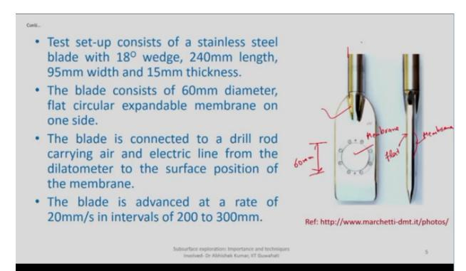
the blade is connected to the drill rod so this assembly whatever you can see on the top that will be again mounted on some drill rod by means of threads, so more and more drill rods as you go deeper and deeper very much similar to your CPT test you keep on adding more and more number of drill rods here.
