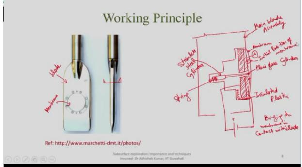
you started applying some section pressure so that the membrane will move towards the blade, so what will happen when it comes in contact with the blade it will become almost in contact with the blade and then in that case it will touch this sensing disk, so this is called as sensing disk.
