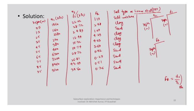
So to start with the problem let's first of all write what are the values given here. So you can write here depth given in meter then the values of Qc given in I am going to write the value directly in KPA because the value of Fs is also given in KPA. So you can write here Fs KPA is I have given here also QF, then the values of we are trying to find out how much will be the value of FR and then based on the value of FR what will be the soil type.
