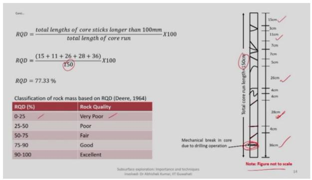
so as suggested here also 0 to 25 means majority of the rock core will consist of small, small fragment, so none of them because it is intact or in smaller, longer length so it will be considered highly weathered rock kind of thing.
