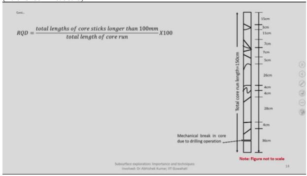
this is you can consider this entire rock core as 150 centimeter is that total length of the core you had actually drilled and brought it on to the surface.
