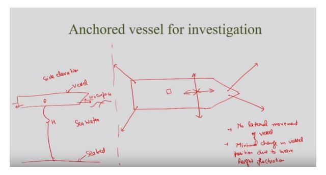
So anchored system mentioned here as like suppose this is your vessel which is generally used for investigation which is actually it's like if I see here it's like something like this which is available in the seabed I mean floating on the sea floor or sea surface or this is mean sea level this is vessel and this is your depth seabed. Now you are interested by means of vessel which is everything filled with water sea water. So, every time you collect a sample minimum this depth
