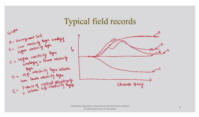
So typical field record, as I mentioned earlier also, so depending upon the dimension, depending upon the subsoil properties, if I put it here there can be writing here, and this is electrode spacing. Okay so if the soil is homogenous, as I mentioned earlier, because the soil is homogenous, that means the soil is not offering any change in the resistivity or the resistivity of the other material is more or less constant. I am calling it as A, so A is
