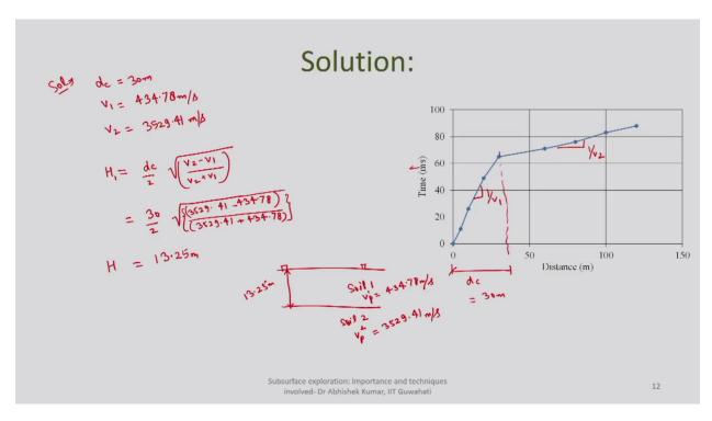
The value of time is giving in milliseconds, so be careful while giving the final values, and then distance is given in meters. So you can simply put those values in Excel and you can get the value of distance time curve.
