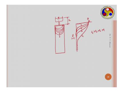
And here if you put realistic values, so, the variation in the water content can be very clearly seen. So, in the particular case what we cloud see that, when soil column and you maintain some certain pressure head. Say you can have your porous plate here and connect to a reservoir, water reservoir you can maintain certain head it could be a constant head.
