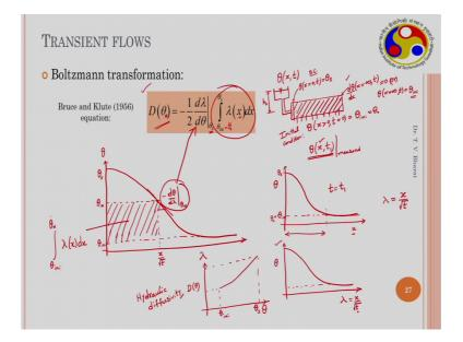
Diffusivity; here the diffusivity is equals to minus half times d lambda by d theta at theta x earlier I would have written theta i that is at given point into integral theta initial value that could be 0 or something theta naught theta naught may be 2 theta x that is it a given point and lambda of x dx this if you solve this here x is a integrational variable.
