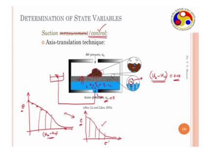
Now, when you start increasing the air pressure, so, u w is constant; maintained constant, may be equal to 0. So, then, you are increasing u a, which is the positive value; that means, this indicates the suction; matrix suction. So, you are actually maintaining certain suction.
