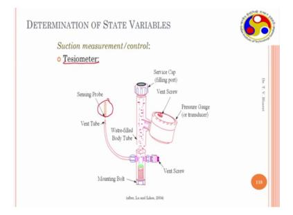
A very common method, that is used in unsaturated soil mechanics, and also in soil science is Tensiometer; for measuring the suction value. This is a popular technique, for measuring the suction in both science and engineering disciplines. And also, this
