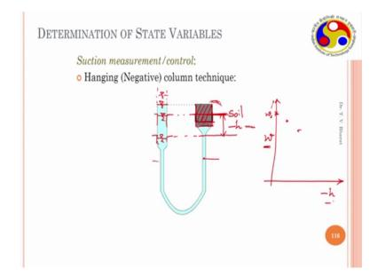
First, the basic technique is hanging column method or negative column method. A pictorial or illustration of the hanging column is given here; where soil sample is placed in a container. You have a porous stone which is attached here, and this is soil.
