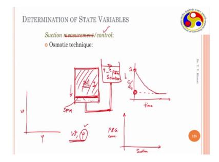
The same technique is used to establish the soil water characteristic curve. So, here you have a soil sample taken in a small column and you put a semi permeable membrane on the top and bottom, or, only just at the bottom. And, you have a porous stone which is placed. So, you have a membrane here and this is a porous stone. So, now, this is, everything is contained in a column. So, this is the soil.
