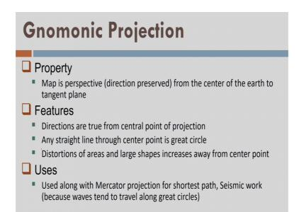
The properties again the map is perspective that is direction is preserved direction from the North Pole that is from the center of earth to the tangent plane ok. So, tangent plane is nowhere it is I put let us say at a I put at the North Pole flat to the equator, parallel to the equator like this.
