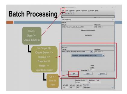
So, that is a batch processing for getting the output. You go to the file, you select the input file which you have recently prepared in the last slide and then you will select your output; that means, in the output you are selecting UTM because you want to project your geodetic 2 dimensional coordinates into UTM map projection x and y fine.
