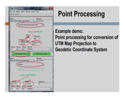
So, you are let us we go back or do the same thing in a reverse fashion; that means, I am converting the point in UTM map projection to geodetic coordinate system. So, what will I do here? I will specify my input in the UTM. These are the further information on the coordinates easting and northing and then I will choose geodetic in the output, then I will do convert upper to lower and it will give me the output coordinates.
