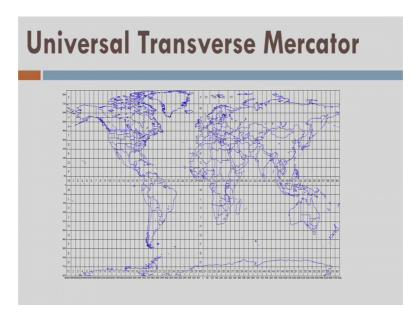
It is a particular type of or the specific example of transverse Mercator projection systems ok. UTM is now most popular map projection system which is being used mostly now, especially including GPS and GNS services, perhaps your map projection system that you are using in your mobile phones or also might be using UTM only ok. So, in this UTM, the picture is shown.
