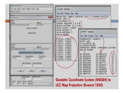
Now, coming to the map projection with datum transformation; so, let us see there is a geodetic coordinate system right and it is being specified in WGS 84 and I am trying to convert into the LCC map projection of Everest 1830, fine. So, we see that input file is there here input and so, I am showing that is this is the longitude information lambda, this is my five information and this is the height information which is of no use.
