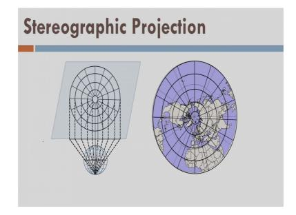
So, of a azimuthal projection where the stereographic projection is there in case of a stereographic projection, I have a light source at the exactly at the South Pole South Pole and it is trying to project the area of ellipsoid above equator and equator. So, there will be a equator that is going to made a circle after projection and all the latitudes or rectangular of latitude above equator, they will be appearing as circles as we can show in the figure ok.
