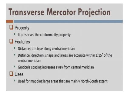
Distances are true along the central meridian ok. Now, you can imagine how nice it is to understand any central, any map projection, distance, direction, shape and areas are accurate within plus minus 15 degree of the central meridian as I already told you.
