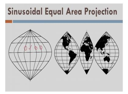
You can see these distorted lines of meridians here and so on, but this central meridian is straight line. So, I expect that the properties along this central meridian should be preserved or they will have a minimum distortion.
