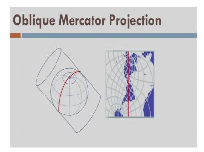
For example, it is see here where the earth is moving here ok. Now, for this Obliques Mercator Projection, I can ensure the same property by tilting the cylinder since tilt cylinder is tilted it is going to cut the ellipsoid, at certain great circle, ok.
