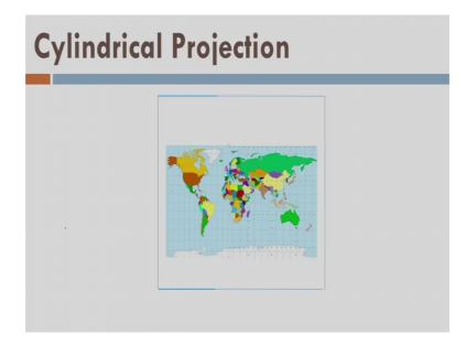
So, since the all the projected points which are projected on the surface of cylinder, now it will open like this like a unfolding of book or rather you are unfolding the cylinders like this. So, this is what is cylindrical projection and which we are doing on a curvilinear surface.
