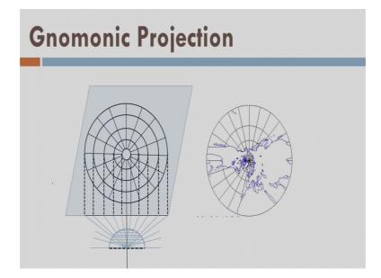
Next is Gnomonic projection which is again a planar or a Azimuthal projection here, you see the light source is put on the center of the ellipsoid and as a result, it is not projecting the equator or rather it will project the equator at the infinity. So, that will not be a visible in the map.
