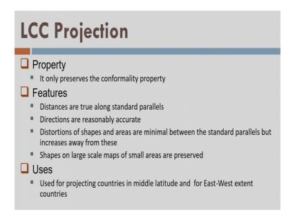
So, directions are reasonably accurate, distortions of the shapes and area are minimal between the standard parallels, but increases away from these. What is a meaning here?
