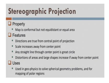
So, this there are some properties; in this map projection, we ensure that this map projection is conformal; that means, deliberately it is ensure that the two lines if they have some angle theta between them the angle between them should remain theta even after projection.
