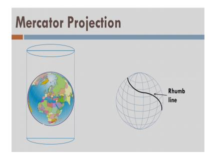
So, there is a Mercator projection shown here; that means, there is a cylinder which is covering the ellipsoid and now I am going to project the ellipsoidal points on to the cylinder
