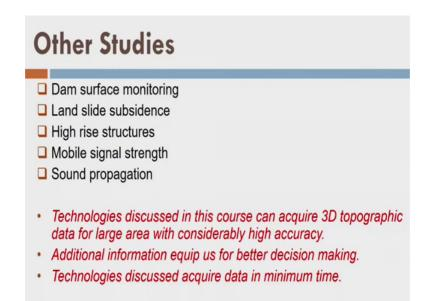
So, the next is the other studies where we can say that dam surface monitoring, land slide subsidence, high rise structures, mobile signal strength, and sound propagation. So, all these studies can be handled with very high resolution data only for example, dam surface monitoring we should use terrestrial LiDAR, we should use photogrammetry. Similarly in case of land slide subsidence even we can see use the RADAR, but landslides should be a regional landslides not the local land slide.
