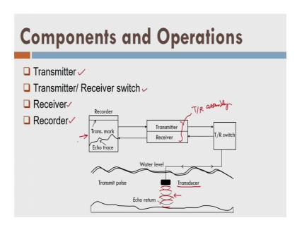
Now, you can look into the operations of the eco sounder. So, it has basically a transmitter or we can say that it has transmitter here as it is shown here the transmitter receiver assembly here, fine. This is nothing but assembly ok now, we have some transmitter receiver switch which can switch on and switch off the operation, ok.
