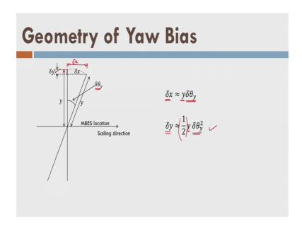
Now, you can see here that the geometry of the yaw bias here it is basically the movement of the vessel in horizontal plane about the z axis like this. So, it is moving like that so, z is not changing x and y are changing, fine. Because of that what happens is here you can see that this position is tracked here or I can see here because of this thing this is the error in the y this portion here and this is the error in the x here from here to here this is your delta x here ok.
