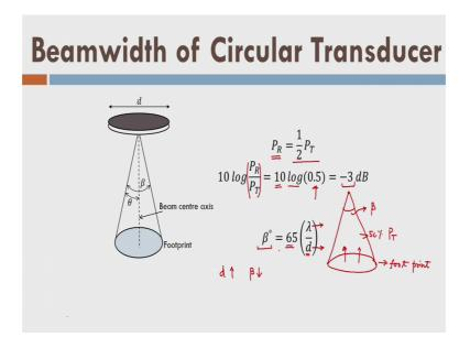
Now, let us consider the beam width of the circular transducer like this, it is my transducer here and there is a depth D. So, it is my cone and so it is footprint, fine, this is my beam width beta. Now, this is the d that is a diameter of the aperture of my circular transducer, fine so, this is my beta bite 2 or theta angle what we call.
