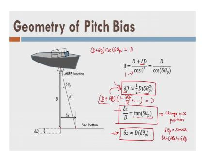
So, from this we can find out that what should be the value of D delta D here because this factor going to be 1 and this factor will be remaining here ok. Now, if you multiply this thing and find out you can find out yourselves that delta D will be equal to the half of the D into delta theta p square ok. Perhaps what you need to do is you need to expand the cause of delta theta p, right in the by the series forms, so 1 minus theta p square by 2 and so on.
