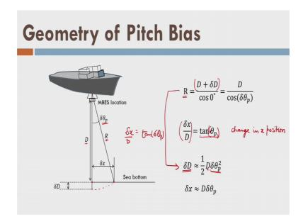
So, let us talk about the error in the pitch what is the pitch here. Let us say this my vessel and vessel moving in the direction of fan here like this the perpendicular to the screen ok. Now, because of the vibration in the sensor because of the vibration in the vessel or because of the vibration caused by the water the vessel is moving like this, right. So, if I say this is my y axis this is my x axis so, right now the pitch is about y axis rotation about y axis, fine.
