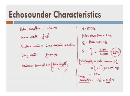
Let us say, first of all I would like to tell that what are the ranges? For example, we have the pulse length or pulse duration in the range of 1 to 50 milliseconds. Then we have beam width it is in the range of 2 degrees to 30 degrees you can see here. And you can compare this figure with the other active remote sensing methods for example, LiDAR in case of LiDAR it was in the milli radians. So, you can compare now the beam width of the acoustic system or the sonar system, right.
