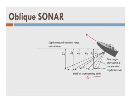
So, this is the figure shown here. You can see that vessel is moving in this direction and in the acrostic direction it is sending pulses up to very large range, right and it is trying to measure the depth like this.
