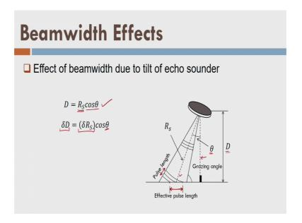
So, let us look into the slide here. So, now, this is my depth D here and by some reason the transducer is tilted with some angle theta which is shown here. So, this is the center line here ok, fine and this is the center line of the tilted pulse ok. What will happen here? You can see that this is your pulse length marked here, fine which is the giving with the resolution and that will be if I make it horizontal that will cut here and here.
