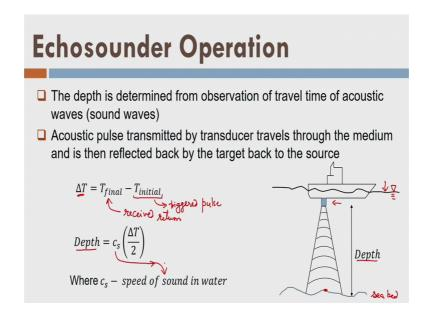
And let us start with the basic concept of the echo sounder. So, the depth is basically determined from the observation of travel of travel time of the acoustic waves or the sound wave. That means, if I have a instrument that is transmitting the sound pulses of sound wave what happens here. Let us say there is a water level at the bottom of the vessel we have mounted an instrument.
