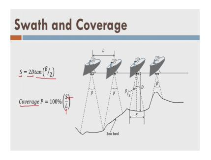
What is the swath? Remember in case of LiDAR we have defined swath as the number of pulses fired across the field of view. In this case since we are considering the echo sounder that is sending only one pulse at a time and so it sends in one pulse the pulse interacts with the ground surface comes back, so pulse interacts with the seabed surface comes back and it is received by the receiver. After receiving it sense in the next pulse, fine
