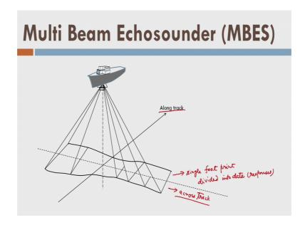
So, let us talk about the multi beam echo sounder. What is multi beam eco sounder? Ok. Remember we have said that if there is a single beam echo sounder what we call SBES it will be sending these sound pulses vertical direction once one at a time. So, it has some limited capability in terms of frequency that is number of pulses fired in 1 second.
