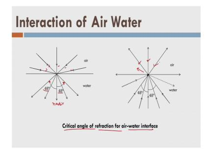
So, here the critical angle of the refraction for the air water interface has been shown here. Now, what happens is that all these pulses are coming here like this and then they are entering into the water with maximum angle of 48 degrees from the nadir here ok. Again the responses are reflected back and again they are converted coming from this 48 degree angle and again going back to the sensor and that is shown here like this, fine. So, that is the idea here ok.
