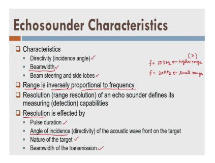
So, now let us look into the characteristics of the echo sounder. So, first is this the directivity; directivity means at what angle it is directing the pulse towards the free
