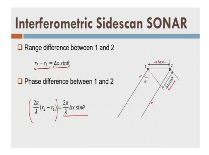
Let us say there is one pulse which is having an incident angle of theta and there is another pulse having the same incident angle. Now, it is pulse number 2 is reaching here, pulse number 1 is reaching here and there is a horizontal distance of my delta x here, fine. So, now, you can see here that this is the difference of my range, fine so, r 2 minus r 1 is this one.
