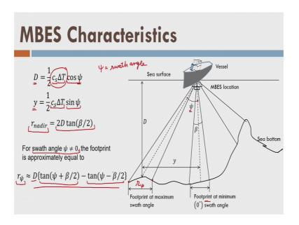
So, the depth is given by at angle of tilt let us say this is this here. Now, I am taking the this another direction so, some this center of nadir direction to this is my psi angle. So, at this psi angle the depth is given by this where it is my travel time delta T and cos of psi, fine because this is the depths here you can see and the we measure the range and range is this quantity ok.
