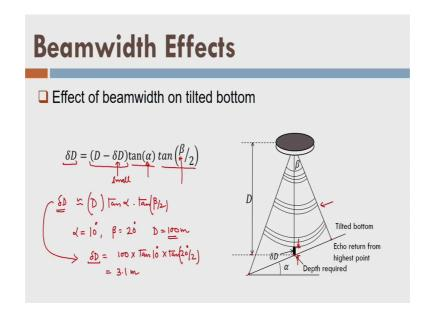
Similarly now, if the transducer is vertical but transducer is positioned very correctly at the bottom of the vessel, so let us assume that transducer is placed at correct position at the bottom of the vessel that means, it should throw the vertical pulses only in the direction of gravity. However, the bed is tilted at angle theta or at angle alpha with respect to the horizon, right so, what will be the effect?
