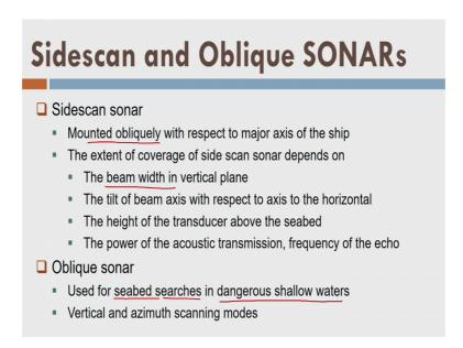
So, what happens is it is the sounder is mounted obliquely with respect to the major axis of the ship there. So, the extent of the coverage of sight depends on the beam widths in the vertical plane. That means, what is the beam width here in this plane which is vertical plane here, fine the tilt of the beam axis. So, what is the tilt here basically?
