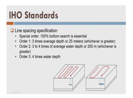
Ok, what about the line spacing? Fine, in case of special order we have 100 percent bottom search which is essential that whatever accuracy we maintain or whatever line is spacing the maintain in case of special order survey, I have to have exploration of 100 percent bottom; that means, complete sea bed or river bed has to be checked. In case of
