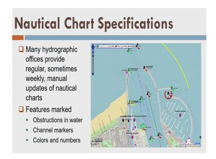
So, once we collect the hydrographic data or by hydrographic survey, what do we do with data? We develop the nautical chart. So, what is nautical chart? Ok so, nautical chart a specifies obstructions in the water and channel markers and it uses different colors and numbers. So, we will see this a specification now.
