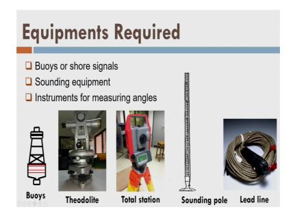
So, what are the equipments required bios and shore or shore signals; that means, there are some signals which are floating in the water and where we measure our xy position as well as depth. So, these are called bios and here it is indicated ok. For the angle measurement we have theodolite, what the total station? Also now they did it is used, because we can measure the distance as well as angle with the total station.
