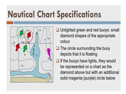
Ok, what next? We have the unlighted green and red buoys to that is small diamond shapes of the appropriate colour. So, these are my small diamonds; that means, the red is indicating the red colour bios and the green is indicating the green colour bios, fine.
