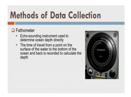
So now we have the fathometers or what we call echo sounders, originally there named fathometers, and now the days we are using the term echo sounder. What it does? It basically sends some sound waves into water surface, and that sounds waves interact with the surface of the seabed or the riverbed and it reflect back the energy of the sound, and again it is collected by the instrument.
