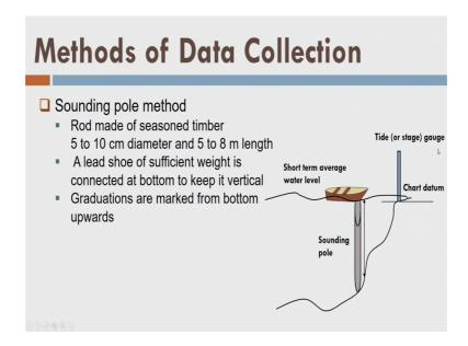
Now, second is sounding pole method. So, instead of rope now I am using a sounding pole, which is 5 to 8-meter length and it is having 5 to 10 centimeter diameter, ok. What I am doing? I am again approaching the bios, that moment I reaches to bio at the x y location or at the position of bios, I will just drop down pole which is called sounding pole vertically down ok. I assume here that there is no water current.
