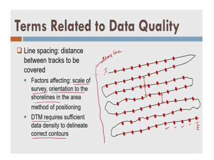
So, once we conduct the survey what do we do? Basically we take a vessel, now (Refer Time: 43:19) the vessel along a straight line ok. During that straight line we observe the points at regular interval, a regular time interval or regular distance interval whatever, fine. So, this is shown here, now you can see here because of the variation in the current velocity, or variation in the boat we are having lines which are not straight, but still we are trying to maintain them.
