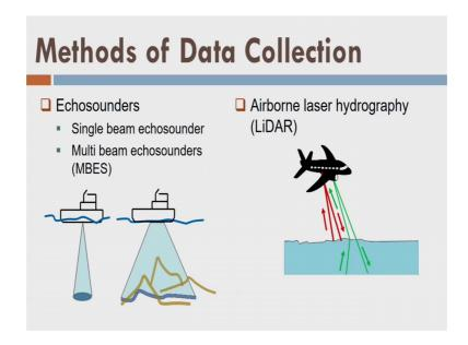
Then we have the eco sounders as we told, then we have the single beam echo sounder. Means, it throws the sound pulses vertically down towards the surface. Then we have multi beam echo sounders, which throws the pulses in the across the track manner, remember? Like LiDAR or in case of radar we have the same mechanism what we call of this broom mechanism.
