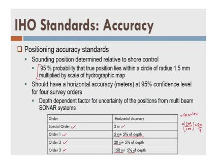
Let us go ahead, now what about the positioning? So, we want to discuss about the positioning also, we determine the sounding which is nothing but depth ok, at the same time we determine the xy position; where we are determining the sounding position.
