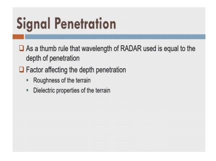
So, first is the roughness and another is the dielectric property alright. So, the rule of thumb is very simple that the wavelength the depth of penetration is generally limited to the maximum 1 lambda or the 1 wavelength of the signal.
