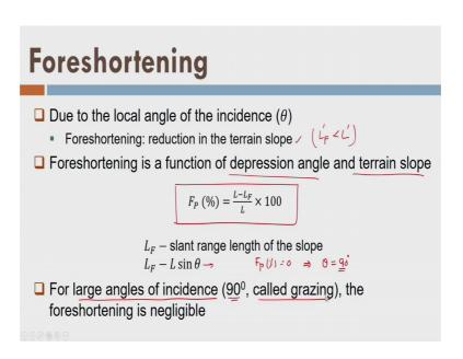
So, foreshortening happen because of the local angle of the incidence or it is nothing but the reduction in the terrain slope ok. So, foreshortening is a basically a function of a depression angle and the terrain slope here ok. So, it will reduce the terrain slope because the length L is represented by LF, L dash F for LF and it is less than I dash all right. So, as a result what will happen the slope of the terrain will be reducing?
