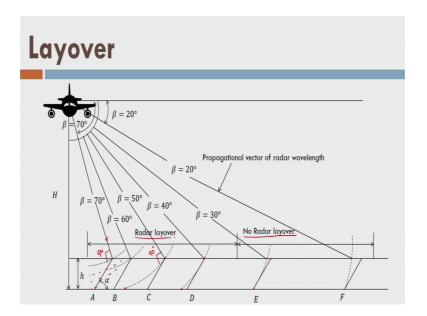
Now, coming to the next phenomena called layover ok. Layover is just like a relief distortion in photogrammetry, but here the relief distortion is completely different aspect and we should understand it first. So, let us see that all some surfaces are there which are shown here, let us say point A, point B, point C some features are there all features are inclined at angle alpha. Now so here you can see that the wavefront is coming and so this angle is my 90 degree alright.
