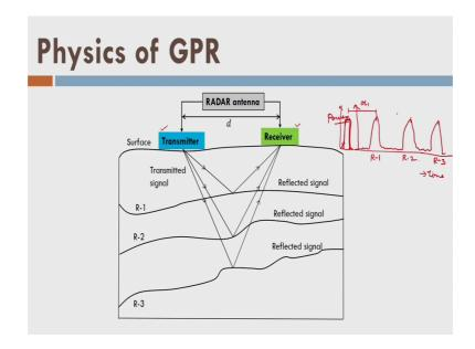
So, let us see what is the simple principle of GPR, GPR here is let us say there are 3 reflecting surfaces R 1 R 2 R 3, which means all 3 layers are low conductive material as well as they are highly reflecting, they do not have the any moisture so I assume all ideal conditions.
