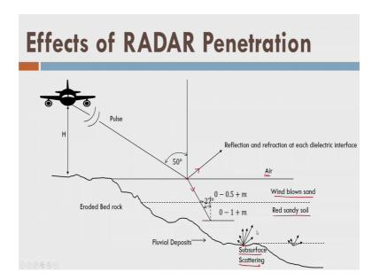
Now, you can see that there is a RADAR pulse and it is interacting or it is transmitting through air and it is interacting here with the surface ok. And it is nothing but the wind blown sand and here this is the red sandy soil here.
