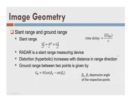
Now, you can see here that distortions will be hyperbolic as it increases with the distance in the range direction, and the ground range which is given by this here ok. So, they are beta 2 and beta 1 are the depression angle of the respective points; so that is my beta angle here.
