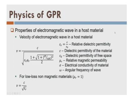
Now how do you use the electromagnetic property of the material or what we call host material ok? The velocity throughout the material of the microwave pulse is given by c is my speed of the light and these are the electromagnetic properties all right, but in case of low conductive material this factor is 0, all right and permittivity is equal to 1 here fine.
