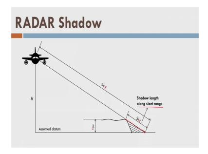
Next phenomena is my RADAR shadow, what is the RADAR shadow? A simple figures show that let us see this is the point here and that has elevation H with respect to some datum because of interaction of the wavefront at this point, this complete length here to here up to this point. This area or we can say this volume will be of the terrain will be under shadow right. There will not be any data from this point to this point on the surface of terrain.
