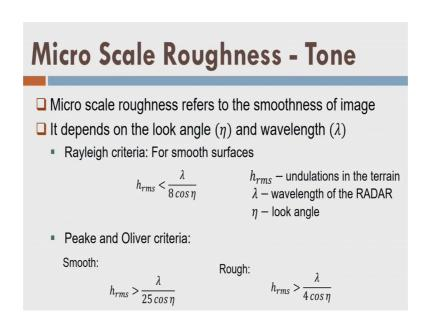
Now let us go into the Micro scale it is referring to the smoothness of the image and it depends on the look angle eta and the wavelength lambda, and it is given by this one remember h rms is nothing but the root mean square value of the terrain variation all right.
