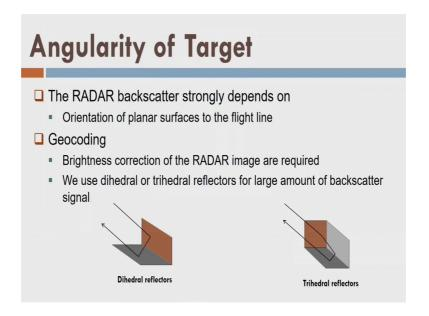
Now, one more aspect is there that is again important from the geometric perspective or the geoscience perspective that is the Angularity of the target, what is the meaning of Angularity right. So, let us see it is orientation of the planar surface to this flight line all right. Now you can see here that in case of geocoding; that means, when the geo reference the RADAR image or we reference the RADAR image in the some kind of object coordinate system or some kind of terrain reference frame.
