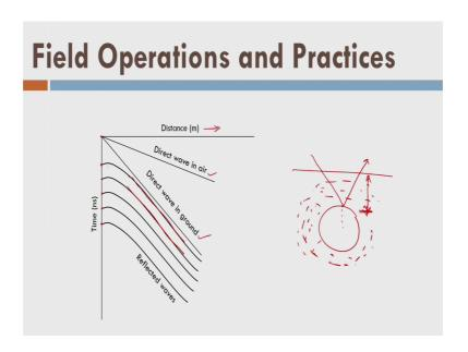
We can see here this thing that as we grow in the distance the between the transmitter and receiver, what happens? First we receive the direct waves and as we are increasing the distance the direct wave also taking the time and that is why this curve is there all right.
