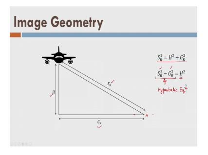
This is my slant range and by Pythagoras theorem I can write the relationship between ground range and the flying height with slant range. So, this is the relationship from this triangle.
