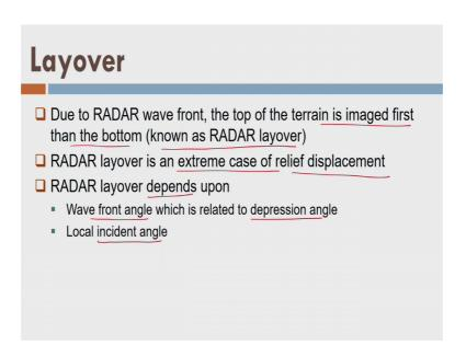
So, due to the RADAR wavefront the top of the terrain is image first then the bottom and this is known as RADAR layover ok. So, RADAR layover is an extreme case of relief displacement alright, but the relief displacement is different from the photogrammetry. In case of photogrammetry if you recall that if this is the line of sight what will happen, relief displacement would have happened on the right hand side not only left hand side well.
