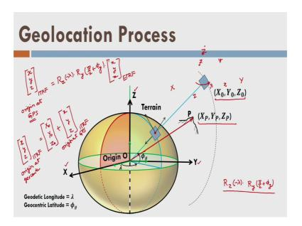
So, I can write here the first rotation is about here right we have rotated about the Y axis ok. Now we will rotate about the Z axis and such that this X axis will be aligned this is your x axis this also y axis before axis is after rotation and this is z axis right this is x axis here capital X here this x axis is same and now Y axis here and now we can see that this angle here is nothing, but lambda fine ok.
