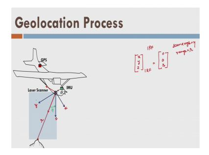
Now, the first step of the geo location process is to convert the instantaneous reference frame located at the scanner, which is acquiring the laser pulses in to the scanner reference frame which is also located at the laser scanner ok.
