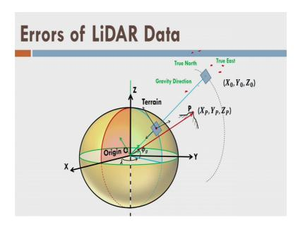
So, I got the coordinates of point P with respect to this reference frame which is green, but located at the geo centre and what is the purpose of this thing. We want to analyse the error in the green reference frame, but located at the geo centre for each and every point this reference frame will be changing because, for each point we have different trajectory points and each trajectory points as different direction of true north, true east and gravity ok.
