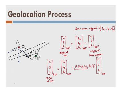
Let us go ahead and now ok so, before sitting on the IMU we would like to convert or we would like to translate our body reference frame, which is located at the scanner to the GPS because, GPS is measuring the aircraft trajectory right.
