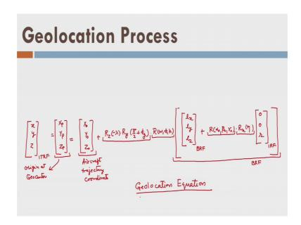
So, the x y z in ITRF where origin at geo centre or I can write here xp yp zp equals to x 0 y 0 z 0 plus R z minus lambda Ry pi by 2 plus phi g ok, what next then we have rotation by omega phi Kappa and then we have the observations in body reference frame.
