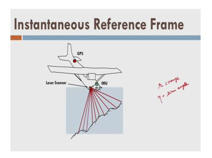
And you can see that there is an aircraft and aircraft is mounted with the laser scanner IMU and GPS fine ok and we have already discussed what is the role of IMU and GPS? GPS determines the trajectory of the aircraft ok. And it acquires the data at every one second between that 1 second we take help of the IMU which measures the role which and your with respect to the true north, true east and the gravity direction ok.
