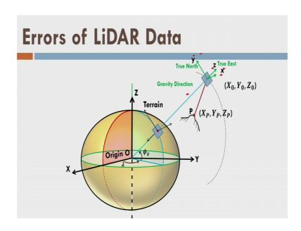
Now we flip the Z axis like this and X and Y axis; that means, my Y axis come to the north axis X into the true east and Z in the opposite to gravity direction. So, it is an orthogonal reference frame located at the aircraft trajectory ok, now let us translate it like this.
