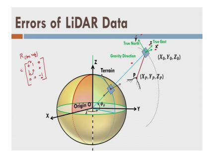
This reflection as well as transformation I can write by this matrix, let us say R inclination and reflection is indicated by this 0 1 0, 1 0 0, 0 0 minus 1 here you can see that I am changing my x to y and y to x here and as well as we are flipping over the z axis by minus 1 right. So, and then we are doing the translation by the X0, Y0, Z0 like this. So, let us write the equation which you have modified.
