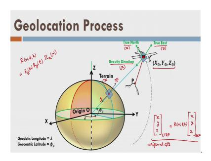
So, let us see that GPS is measuring X 0, Y 0 and Z 0 coordinate of the aircraft trajectory here, shown by the red colour there right ok, Now let us define the earth tangential reference frame, which is we have already defined this is my local geodetic horizon and I have defined again here.
