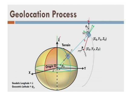
And now I want to bring this earth tangential reference frame into the geocentric reference frame. So, now, you see this is your Z direction here is Z direction and what is the angle here this is your phi g angle which is written here ok. So, total rotation between the Z axis this Z axis of ETRF and this Z axis of the ITRF is equal to 90 degree plus phi g ok. So, let us do the rotation here like this ninety degree and then this 90 degree plus phi g. So, that is my Z axis is aligned now ok.
