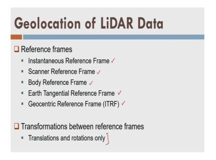
Now, in order to understand the geo location process, we need to define some reference frames ok. So, we have five reference frames here and that will connect our basic measurement of the laser pulse to the ITRF reference frame. So, the first is instantaneous reference frame, then we have scanner reference frame, then we have body reference frame, earth tangential reference frame and finally, geocentric reference frame or international terrestrial reference frame ok.
