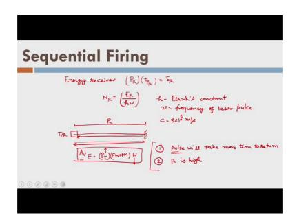
So, what about the energy at receiver? Let us say there is a pulse which is reflected and which is having P R as a peak power and if we say that the t p is a pulse length of the received pulse. So, that is my total energy of the received pulse fine, ok. What about the number of photons of the received pulse I can find out E R divided by h nu, where h is plank constant and nu is the frequency of laser pulse, ok. Now, what happens here let us
