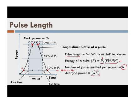
And, now we can say that what is the energy of a pulse is equal to the peak power into FWHM; that means, energy content within a pulse is equal to peak power peak power into pulse length, right. So, now, I have approximated my laser pulse which is normally distributed by a rectangular box. It is easy to deal or make any estimates with the rectangular pulse now.
