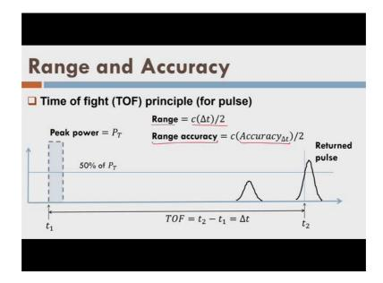
So, let us further what is the range and accuracy as I already told the range is c times delta t and. So, we have the accuracy of the delta t and that is the time measurement that decides my range accuracy or the resolution of the laser pulse.
