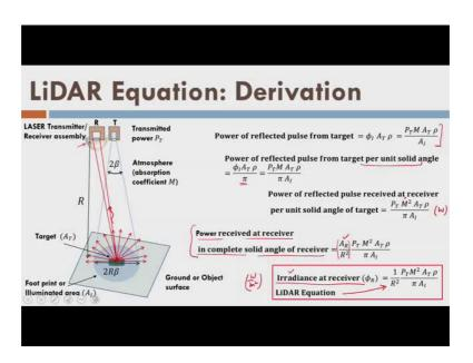
Again coming same thing, right. So, this is this, ok. Now, if I assume a hemisphere around the target we can say that in the solid angel the unit solid angle of the hemisphere how much energy or how much power is being reflected by the target. So, this is the power reflected by pulse in the per unit solid angle of my target because we are dividing it by pi which is a solid angle of hemisphere, right.
