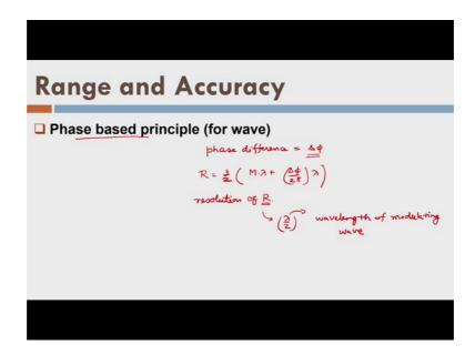
Similarly, if I see in case of phase based principle the measure the phase difference equal to delta phi and we right one think here that distance is R is given by 1 by 2 M number of cycles so, M lamda plus two phi into lamda, that we have already seen in case of total station and the same expression I am writing here.
