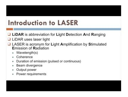
So, LiDAR is an abbreviation for Light Detection and Ranging ok. LiDAR uses the laser light, ok. Why laser light? So, let us first try to understand what is the LASER and how is it useful in order to do the ranging and detection, ok. So, LASER is an acronym for Light Amplification by Stimulated Emission of Radiation, right. So, it has some certain characteristic like wave length, coherence, duration of emission, beam divergence, output power and power requirements.
