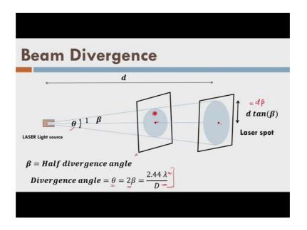
So, now we see there is a laser light source and it has some opening and because of that opening the laser light is deflecting at the corners of that opening and as a result it will create and spot or it will illuminate some area not a point it will illuminate some area on the object surface which is this. Let us see how does it do. So, this is distance d the from the laser light source and the object surface and now, this is spot is created by the laser
