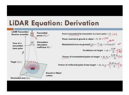
So, that is my transmitter here and it has some aperture there is range R. So, this is the illuminated area and this is my laser spot which is shown here by illuminated area and we also call it footprint, this is cone of the transmitted laser pulse, ok. So, now, this is my divergence angle 2 beta, ok. So, we have 2 R tangent beta as my foot print or laser spot diameter. Well, we call it footprint in case of topographic mapping ok, right. So, I can approximate it by 2 R beta, fine.
