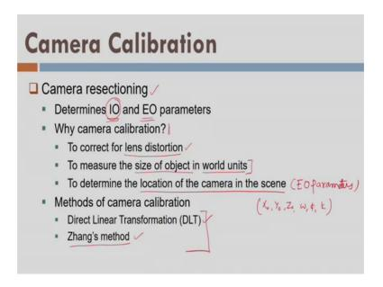
So, the camera calibration as we have already talked is all about finding out the interior orientation parameter of the camera. Now so, I want to determine I O parameter basically; however, in a whole process we also determine their E O parameter.
