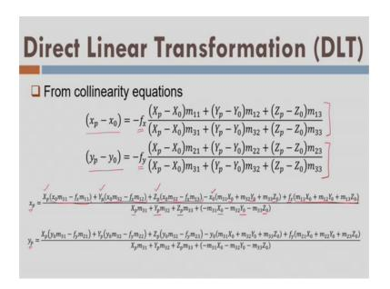
So, let us start with the Direct Linear Transformation or DLT method ok. On the screen I am showing you that 2 equations, which are nothing, but collinearity equation that we have proved it ok. So, I have rewritten these 2 collinearity equations, where you can notice that there is some difference here; f x and f y; that means, I am assuming that the focal length in x direction and focal length in y direction of the camera image are
