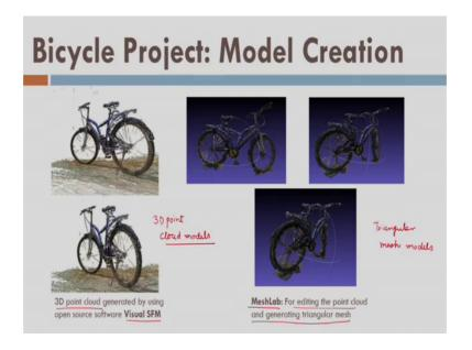
So, 3 D point cloud generated by software called Visual SFM which is free. And, these 3 more models that we have further we use the 3 D point cloud generated by the SFM visual SFM software and then we have done some kind of processing over there using MeshLab software and that is also free. So, then we have done the editing and generated the triangular mesh. So, these models are triangular mesh models and these are the point cloud 3 D point cloud models.
