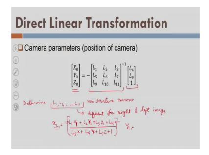
Finally, the 3 D coordinates of the camera position for left image as well as right image. So, now, you use these equations and you can find out X 0 Y 0 Z 0. And, that is the most elegant part of the DLT that first of all you are determined all parameters L 1 L 2 L 11 without iteration or it is by non iterative manner.
