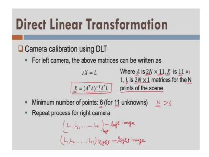
So, once you determine this X values then you can straight away in a single iteration you can determine all 11 parameters ok. So, how many points do I need as a control points, there are 11 unknowns and if I take 1 point it is giving me 2 equations 2 collinearity equation or 2 DLT equations. So, using 2 DLT equations I can find out 2 set of conditions. And, hence for 11 I need minimum 6 points, because the 6 points will give me 12 equations.
