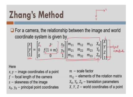
So, as a result I know the dimensions of my checker board and I know what are the control points right. With the help of some image mating technique and with the help of let us say some algorithms like shift that is scale invariant feature transform. These points which are called control point in the object can be identified automatically. And, as a result now the camera calibration process becomes completely automatic, because of the image identification or the feature identification number 1.
