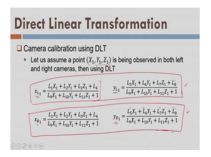
So, let us assume that there is a point X 1 Y 1 Z 1 is observed in both images. So, now, I can write this equation; these 4 equations I can write easily right and I have already modified my equations the collinearity equation in the form of direct linear transformation equations. So, this for left image I have these 2 equation, for right image I have these 2 equations. And, remember these parameters are different from both left and right images.
