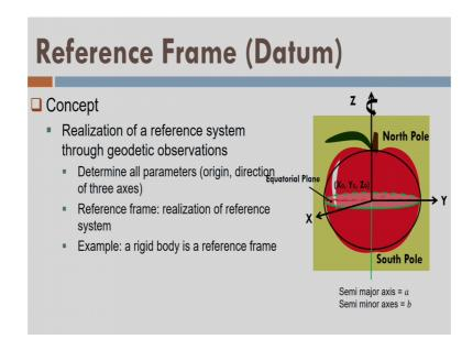
And this is my rotation axes and rotation axes is cutting at north pole and south pole and remember that if I fit the geocentric system; that means, the origin at geo center of the earth and the rotation axes is completely aligned with this thing, I can understand that it can be a global system. Let us look into detail of this thing
