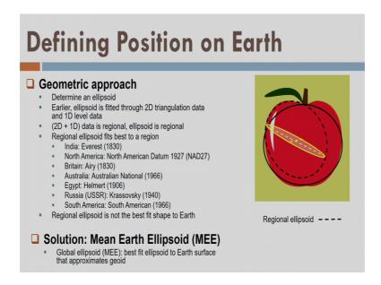
Geometric approach says that let us fit an ellipsoid which is a geometric figure on the given surface of the earth ok. And we have already discussed that we have some reasonal ellipsoid which are already fulfilling the local purpose of a particular continent or particular country or particular region.
