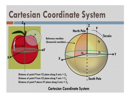
This is my cartesian coordinate system for the earth. So, let us say point P which is zoomed here. So, now, for point P, I am drawing a Z P X P and Y P. So, this is my cartesian coordinate system and I am defining the cartesian coordinate system for the kind of geodetic or geocentric reference frame for the earth.
