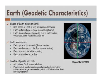
So, now let us look into the shape of the earth. So, what are the earth characteristics because of that we want to develop our strategy or methodology in, so that, we can develop a 3D reference system in which we can measure our 3D coordinate simultaneously. So, this is the surface of the earth as visible from the satellites. And now, if we say that the real shape of the earth is very irregular and complex, as we can see
