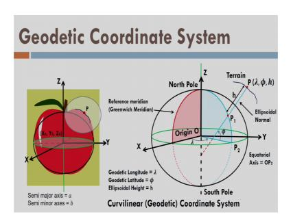
So, I have a geodetic longitude here lambda geodetic latitude phi and ellipsoidal height h; well this kind of figures are available in the book.
