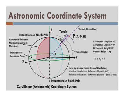
What about the role of ellipsoid here? So, far we did not find any role of ellipsoid. Although, we are showing it here for the purpose and the purpose is the height between the geoid model and the ellipsoid is called geoidal undulations and represented by N g. Well, and earlier we assumed for a regional ellipsoid that, the regional ellipsoid the line vertical line and the ellipsoidal normals are parallel or they are basically the same and
