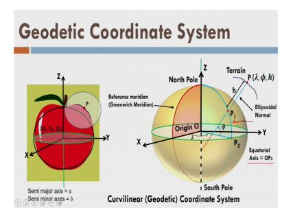
Let us draw a perpendicular from point P to the ellipsoid that we are dropping a perpendicular from point P to the ellipsoidal surface. So, this is the perpendicular and this is the intersection point of ellipsoidal surface or ellipsoid with the perpendicular line from point P. Now, if I extend the line perpendicular line to the equator, it will cut here and now, if I further extend, it will cut the rotation axis of the earth.
