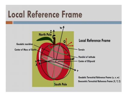
So, we are showing here a geocentric terrestrial reference frame X Y Z and geodetic terrestrial reference frame u v w here, ok. What about the local reference frame? Well, again we are showing a geodetic reference frame and a geocentric reference frame in this
