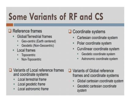
Now, finally, we can see there are some variants of reference frame and coordinate systems. For example, we have reference frame global or terrestrial reference frame, then we have local frames in case of global or terrestrial frames, we call it geocentric or geodetic in case of local reference frame, it is called topocentric and non topocentric. Remember, if the origin lies on the surface of the earth of a local reference frame, it is
