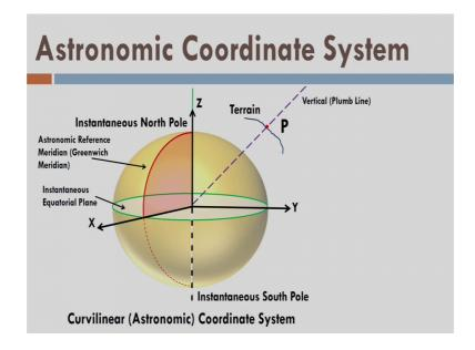
Let us go to the astronomic coordinate system. Here in case of astronomic coordinate system, again point P is same, but let us define the plumb line or the vertical line, that is called vertical or sometimes called plumb line in literature, that is the line of gravity passing through point P. So, it is going to intersect the geo center of the earth and that is why, we are straight away drawing it to the geo center.
