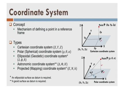
Now, coming to the coordinate system, a coordinate system is a mechanism of defining a point in a reference frame. Remember, we have already defined reference system and we define realization of a reference system is a reference frame. Let us see, I want to measure a point in 3D.
