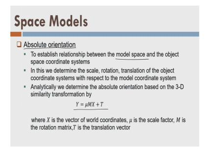
One is absolute orientation; that means, using bundle adjustment or using space resection and intersection. We have calculated the unknown coordinate parameters; that is X P, Y P, Z P in object coordinate system. And now you are ready with the lot of 3-D coordinates you can develop a 3-D model. So, let us see that you have a 3-D model using 2 images only and another set of image is there; which is give you another model 3-D model and you want to orient these 2 models together.
