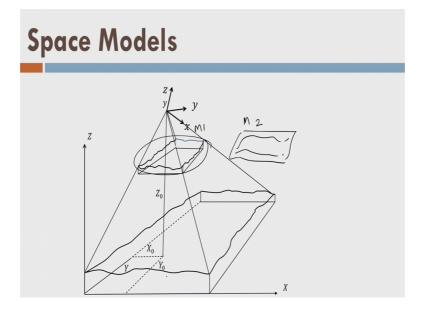
So, it is specified here like this, this is a 3D model here shown here and I am bringing into this coordinate system there could be another 3D model here like this and I am bringing model 2 and model 1 both into this coordinate system capital X, Y, Z. So, that is what we call absolute orientation.
