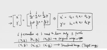
First of all let us do some revision because we want to use the computational photogrammetry or the analytical photogrammetry or the numerical photogrammetry. For that we need to understand some of the concepts like least square solution and for that purpose let us revisit the affine transformation as well as solving the affine transformation by least square solution. Especially we are going to use observation equation method.
