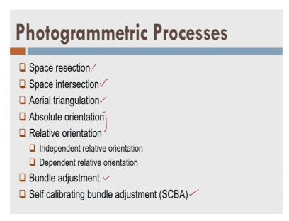
Now, in this lecture we are going to learn space resection, space intersection, aerial triangulation, orientation absolute and relative and then we are going to talk about the bundle adjustment and self calibrating bundle adjustment ok.
