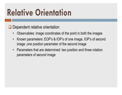
First is dependent relative orientation, means all the one is becomes my reference and another becomes my target or slave and that is now moving like this. So, that is called dependent relative orientation, where we have aligned one image with respect to another image and then we have created the 3-D model.
