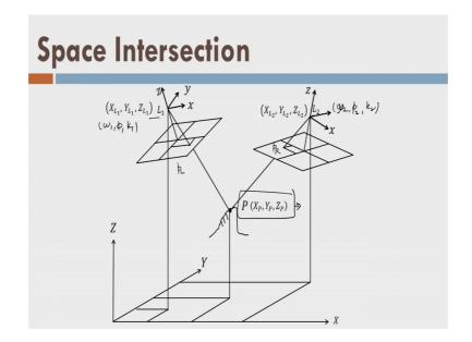
Yes, in case of space intersection what do I want to find out. I know; what are the interior orientation parameter for a camera, I know what is the exterior orientation parameter for a image like this. So, there are 2 images, I know they are exterior orientation parameter which means I also know omega 1, phi 1, kappa 1, I also know here omega 2, phi 2, kappa 2 now but I do not know coordinates of point P and I want to find out the coordinates of point P.
