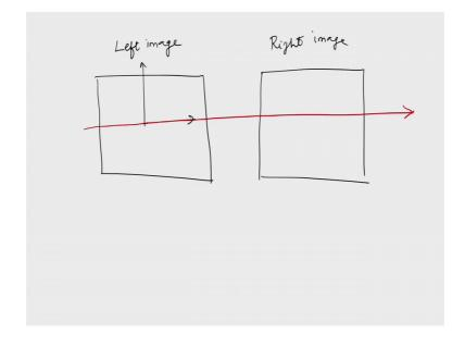
So, that 2 images 1 is left image call it left image and the right image. Here, in the all derivations we have assumed this is my flight line like this is my x and y axis or this is the flight line from here like this; that means, here I assume that I have already aligned the flight line of the 2 photographs, which are consecutive acquired in a same flight.
