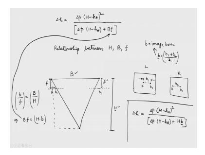
So, we expressed the height difference between the 2 points delta h as delta p, H minus h A, square divided by delta p, which is difference of the parallax of the 2 images for the 2 points like this ok.
