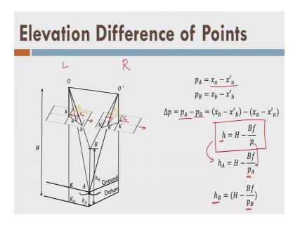
So, let us start again now I want to find out the elevation difference of 2 points. So, I have already shown you how to calculate elevation of a point. Now, I want to find out the elevation difference and there is a advantage that will see now. So, let us see there is a datum and there is a ground and there is a point A, which is height h above datum now point B is there which is exactly above the A and this has height h B.
