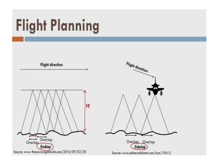
Here, before we start we have to understand one thing that let us see there is a flight and it is flight is mounted or the airplane is mounted with an camera. So, instead of creating 2 camera; that means, for stereo vision I need to have 2 eyes or maybe 2 cameras. So, what will I do now I will put one camera only one camera on a flight and then the airplane will move in certain direction.
