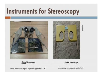
So, this is the instrument what we call as stereoscope. We have 2 type of stereoscope: one is called mirror stereoscope, that you put 2 images and remember that 2 images are aligned in a way that flight lines; that means, if I go back to slide last slide. That is blank slide.
