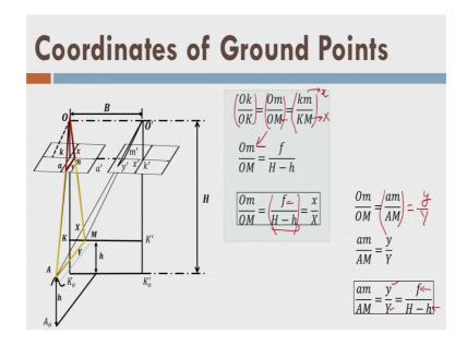
So, in order to find out the 3 D coordinates to find out x y and z coordinates. So, let us first find out the x and y coordinates. The moment I find out x and y coordinates, then I will find out z coordinate and then I can say that is ethyl photography is acquiring all the things together, I am developing a simultaneously measurement of x y and z system, but mathematically I am doing separately.
