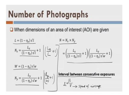
So, let us go to the next slide where I write, this is the effective length covered on the ground similarly, I can write effective width by covered by 1 photograph on the ground ok. So, what about the number of photograph along the x direction along the flight
