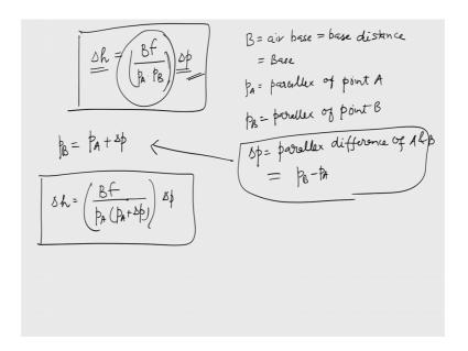
Where I write delta h in terms of parallax difference and parallax values I am writing it as del delta p. So, you see that how the delta h is a function of delta p; that is the height difference is function of parallax difference or I can see if I multiply the parallax difference by this term here I can get the height difference.
