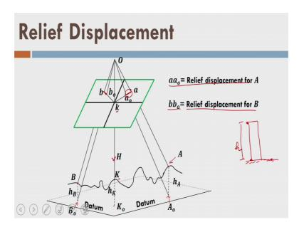
So, let us talk about the some kind of displacement that happens that are evident on the vertical photographs. So, first is the relief displacement. So, let us see there is a datum like this datum surface is this way fine. And, from datum surface if I measure the height h A and h B for 2 points A and B on the terrain so, I will have these points h A and h B. So, they are the elevation from the datum. Now, let us see the B 0 is this point here. And, similarly I have A 0, which is this point ok.
