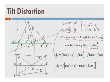
Now, let us try to find out mathematically. What is the amount of tilt distortion? So, this is my focal length in the tilted plane and this is also equal to the focal length in the vertical photograph, because I have finding out what is the equivalent vertical photograph of the tilted photograph right. Now, I can say this is my tilt distortion d a in the photograph in the animation. So, I can write it like this I can also write it like this you can see here that i a dash is equal to this one ok.
