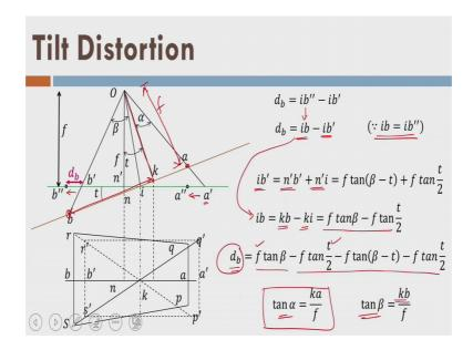
So, what about point b again this is my focal length f. So, let is my distortion db you can see here that because of the tilt distortion point a is shifting inside like this, but point b is shifting outside right.
