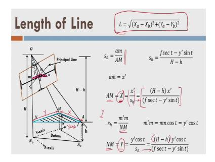
So, length of a line, so let us measure the length of a line on a tilted photograph.
