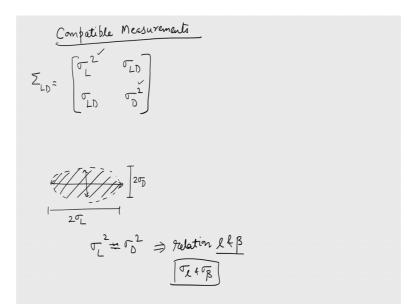
If you remember we have find out the matrix sigma L square sigma L D sigma D square in case of latitude departure example, this one right, as we said it is my sigma L D. Here if you see that if my length measurement is very, very accurate or bearing measurement is very, very accurate and as a result of that I am getting some value of sigma L and some value of sigma D, which are quite different, right.
