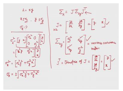
And area is given by x and y as a multiplication of x and y, ok. So, let us see that if x is measured, let us say the length of this room and width of this room x and y are measured with some standard deviation value, ok like this ok, now I want to find out what is the value of sigma A. And that is why I have given a simple formula there, that let us see if I
