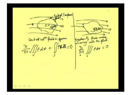
Now, say model of flow one we can, one very popular term here in hydraulics we use is control volume. Say this is one control volume. You can just concentrate into the slide this we use. We are using the, this is a, this is a control volume; we are naming this is a control volume and this surface of that volume we are saying as control surface, control surface.
