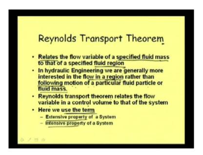
Well, we are not going into much detail of this part, but still I am just considering, I am just trying to explain some of the very fundamental. Well, then you can concentrate again on the slide that Reynold's transform theorem, Reynold's transform theorem, this is also one of the important theorem that we need to know before deriving those equations. Well what it means that Reynold transport theorem relates the flow variable of
