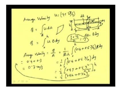
Let me keep the diagram in my front, so that we all can appreciate say this is the expression and this is what we have already drawn, and then, at any point, any section at depth y, this velocity is u; that means, this segment is u and this is d y; this distance is b. Now, what is our average velocity? First, to calculate the quantity flow discharge or mass, if we want to calculate, then we need to know the average velocity. So, let us compute first the average velocity.
