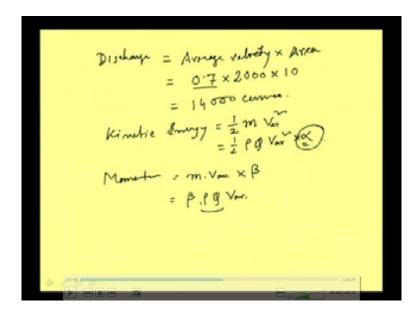
So, we can find out the discharge is equal to say average velocity, average velocity, multiplied by the sectional area. So, that average velocity already we have got 0.7 and sectional area as we know that average which we are considering this to be 2 kilometer. So, it is 2,000 meter and then depth is 10 meter. So, we can find this to be say 14,000 cumec, 14000 cumec, cumec, and once we get the discharge, if we need to calculate mass, here just we need to multiply it by rho to get the mass.
