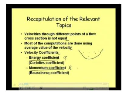
First, we did discuss that velocity through different points of a flow cross section is not equal. What we mean by that? Velocities through different points of a flow cross section are not equal. That is what we did discussed, and by that what we mean that, if this is the
