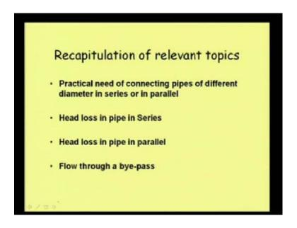
Before going to the pipe network, let us see the in the last class what we did. We were studying practical need of connecting pipes in different, pipes of different diameters in series and in parallel then of course, we did discussed, how we calculate the head loss in pipe in series. And then of course, we were studying how we calculate the pipe loss, the head loss in pipes when they are in parallel and of course, we did refer that parallel does
