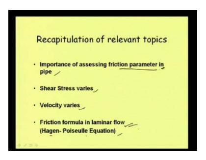
We were stating in the last class with that importance of assessing friction parameter in pipe. Then, we were talking about for, actually in fact to get that particular topic in more detail, that assess the friction parameter, we were discussing on how shear stress varies within the pipe diameter, within the pipe section. And then, we were discussing how velocity varies within the section in a pipe and then with the help of these relationship,
