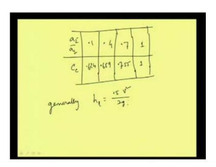
And then, we can have as I said, that we have this sort of ratio say, a 2 by a 1, if we put say, and then we can have the value of c c, there is a 0.1, 0.4, 0.7, 1. 1 means this pipe is not having any contraction. So, if we get this sort of a table and then this table gives that this is equal to 0.624 when it is 0.1, a 2 by a 1, a 2 is the downstream point that one and
