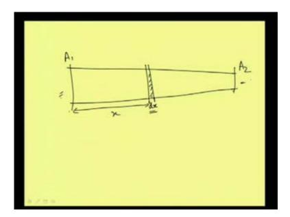
Then there is another issue that, if a pipe itself is contracting like this. If a pipe itself is contracting, tapering pipe. Well, the pipe is tapering and in that case the friction formula
