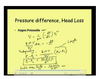
So, this Hagen poiseuille equation, how we can derive, already we have got that v average, now we are writing as v, v is equal to say 1 by 8 mu, then minus d p d x into r 0 square. So, pressure difference now we can just have it in different form and what we can write, that 8 mu v just changing it to this side, 8 mu v and then on the right hand side divided by r 0 square of course r 0 square, then we are keeping the d x here, is equal to
