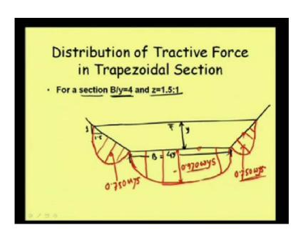
Let us see how this distribution occurs and of course, they did it for different type of channel, different type of trapezoidal channel means say trapezoidal channel with side slope something. I mean may be 1 is to 1.5. They conducted some experiment with side slope 1 is to 2. They conducted some experiment with rectangular channel. So, like that
