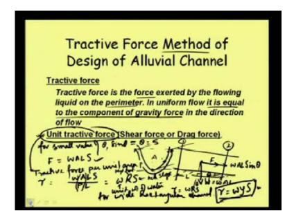
That is why later on people tried to develop one method. Now days, this method is used for design of alluvial channel. In fact, in Indian court also suggest this method that is the Tractive force method of design of alluvial channel.
