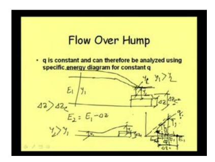
Well, then like this narrow down, sometimes we can have a situation where this depth is raised not depth rather the width is raised, suppose the bed is raised by delta z amount, delta z amount then a sub critical flow is coming then what will happen to this one? Say this is E 1 energy and at this point say what we can write that E 1 or E 2 is equal to E 1 minus delta z, otherwise there is no energy loss that is why we are using, as here we can use the relation, our specific energy diagram.
