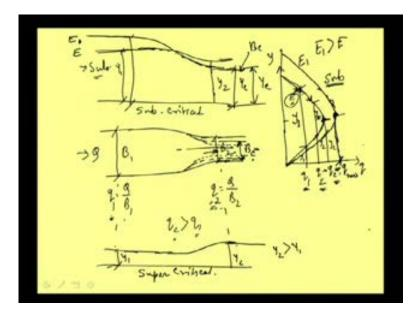
Now, if we just use the value here, say this is my y 1 where q is this one; q is this one we are talking about sub critical flow. So, this is the y 1 this is the y 1 and this is the y 2; q 1 is this one and q 2 is this one well. So, for this sort of situation, we can see when discharge q 1 I mean unit discharge q 1 here is less than the unit discharge q 2. That means, it is the situation of this kind, you can refer the diagram q 1 is less than q 2, q 1 is
