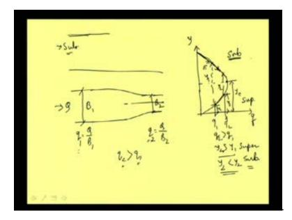
Then now, we can try to analyze the situation when our flow is changing through a when our flow is passing through a width or contraction, channel contraction. Say here our B is B 1 and here B is B 2 well and q coming is q fine. So, unit discharge q at this point is q
