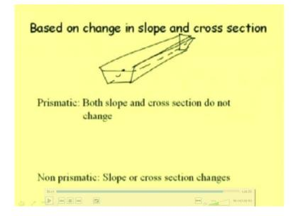
So, if a channel is carrying water and say its cross section here is like this and it is carrying water up to this much depth and this channel is of this type and its cross section here is like this, and say this cross section here and here if it is not changing if it is not changing of course, in my diagram it is, it is, appearing that it is changing, but it is a long distance. That is why it is narrowing down. So, if it is not changing, then we call this as a prismatic channel.
