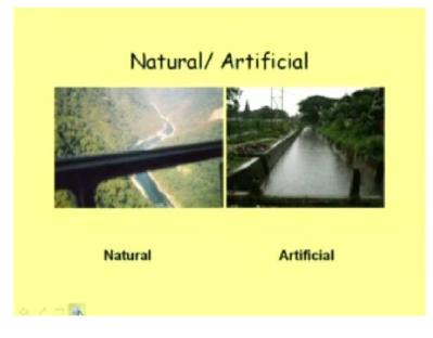
So, like that based on the shape we classify open channel into different classes, and then, again based on whether it is natural or artificial, it is very much known to all of us that a channel existing in the nature we call natural; a channel that we are constructing we refer as artificial channel. Then which is more important is the based on change in slope and cross section.
