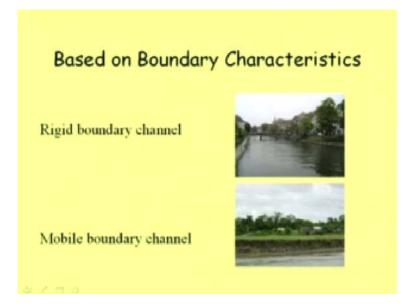
So, both slope and cross section must remain same. Well there is another classification, and then, based on the boundary characteristic, say if we classify we, if a channel is having a proper boundary, then it is referred to as rigid channel boundary which is say non-erodible, and then, if the channel is of this type, then we refer this as a mobile boundary channel; then we refer this as a mobile boundary channel.
