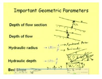
Well, this two terms are important, because in this slide, we will be showing that how these two parameter are used to define some of the important parameter of, I mean open channel flow. Well, depth of flow section, again before going to these terms, let me discuss the depth of flow section. As I was telling this depth of flow section means say as flow section we means always it is normal to the bed.
