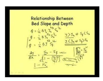
Well, now we need to discuss, so we have covered M1, M2, M3, S1, S2, S3 and C1 and C3 profile. Now, we need to cover two different types of profiles that are four different types of profiles forming over two over horizontal bed and two over adverse slope channel and for explaining that situation where Sb suppose for horizontal slope Sb equal to 0.
