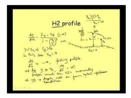
Well, then for H2 profile definitely we will have to use this sort of understanding because this is advantageous here. Well, let us draw one horizontal bed and in fact you may have some equation that when it is horizontal slope, then how flow will be occurring because there is no component of because entire flow that is open channel flow that the governing force or say rather, we can say the driving force is the component of gravity force acting in the direction of flow.
