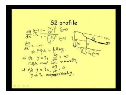
And let us discuss about the characteristic of S2 profile characteristic of S2 profile; here the bed slope S b is greater than S c, the same thing this is normal depth line NDL, and this is critical depth line CDL, and our profile will be here; and let me draw, it as a
