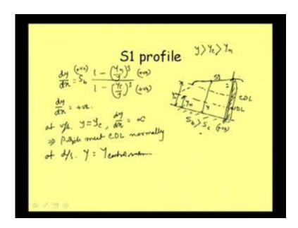
Well, the S1 profile means it is a steep slope like this, and in case of steep slope this S b is greater than S critical slope, and of course positive, of course positive, but it is greater than S c; and when it is greater than S c, then our normal depth line will be somewhere here, say NDL, and critical depth line will be above the normal depth line, this is what CDL. Now, when we talk about zone 1 that means the profile will be here.
