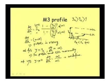
Then let us see we are left it one more profile in mild slope that is M3 profile. Now, in M3 profile say this is bed slope is always mild S b is less than S c, and of course, it is positive, and as explained already this is CDL, and this is NDL, this is NDL, and profile
