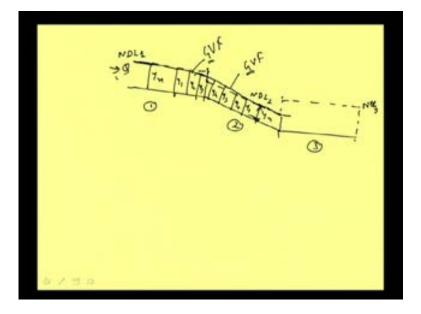
Well, now from our understanding of uniform flow, we had seen till now, but suppose a discharge Q is coming here. Then for this slope, suppose our uniform flow level is this much; NDL 1 suppose in this section 1, section 2, section 3. Now here, as the slope is increasing in the channel 2, as the slope is increasing, so obviously, the depth of flow or
