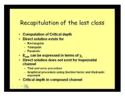
Well we started our last class with the computation of critical depth, well, and while discussing the computation of critical depth, we could see that direct solution to critical depth exists in case of rectangular section, that is when the channel is rectangular in case of triangular section, that is triangular channel, and in case of even parabolic section also.
