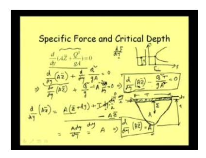
So, that is what we are getting that after increase of depth by dy, the moment of area above the surface is this one, and then change we can get that, this minus area into Z bar, this is for the original, so what we are writing basically d dy of A Z bar is equal to this is the change, and we want to get it in terms of dy, I mean with respect to dy, how much change, it has occurred due to change in dy.
