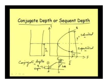
Then, we were talking about this conjugate depth; so, let me just draw the diagram again, and we have already drawn it, that this is the channel section, so the depth corresponding to F minimum, here we are plotting specific force, and here it is y is called critical depth, that is, now you can write here y c.
