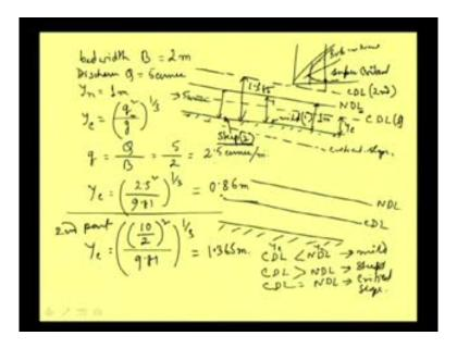
Now, that means, in this problem, if this is not given, suppose, we were given the bed slope of that channel, suppose if we were given the roughness of the channel, then we could have calculate what the uniform flow is, but now in this problem, uniform flow depth is directly given, that is 1 meter depth is the uniform flow depth for a discharge of 5 cumec; now, what they want to know well.
