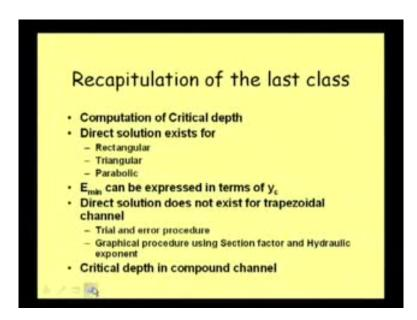
And if we want to go for considering these as a trapezoidal channel, then we need to go for trial and error procedure, and in a trial and error procedure, we need to first consider one initial value, and what will be that initial value.
