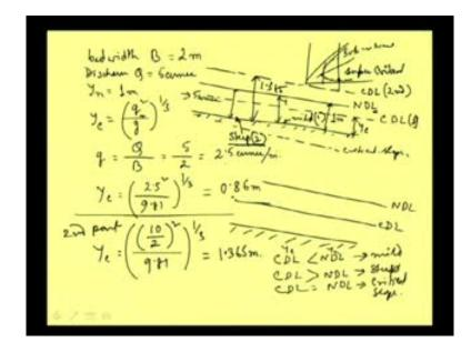
Well now how to check this, the problem though it looks somewhat complicated, but it is not like that, it is very simple one, say in this given problem, our first, we let us mark what are the things, say bed width is given, bed width B is given as 2 meter, and discharge Q is given as 5 cumec, and normal depth y n what we are observing is 1 meter.
