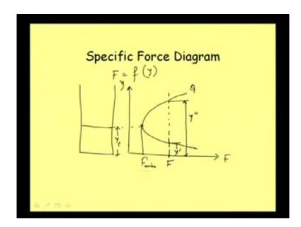
And that way specific force F is a function of y, and if we plot this diagram, this, these two value in a graph, then it will be like that depth y and specific force F, and this diagram will be of this shape, this diagram will be of this shape. And here also, and this is of course, for a particular Q, it is for a particular Q with the increase of Q, again if we change Q, we will be getting a, another curve for different Q, we will be getting different curve well.
