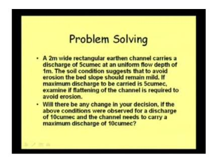
If the bed slope becomes steep, well by mild what we mean, and by steep what we mean, that we did discuss earlier also. If the bed slope become very steep, in fact, it is the steep, and mild are technically steep, and mild that means, we are meaning, that, it is, it is not literal meaning, but it is a technical meaning, that when our slope is greater than critical slope, that we did discuss in our last class, that is when our slope is greater than critical slope, then it is steep slope.
