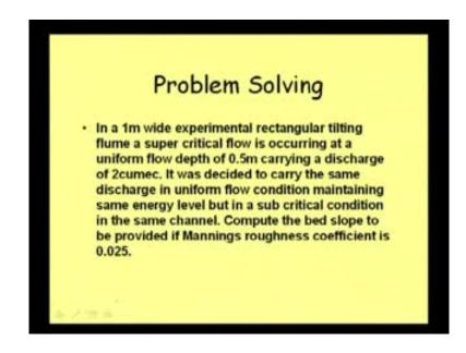
Well, so let us take another problem; in a 1 meter wide experimental rectangular tilting flume, now, we are talking about a experimental tilting flume, a supercritical flow is occurring at a uniform flow depth of 0.5 meter carrying a discharge of 2 cumec.
