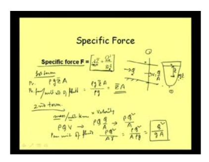
Then the average pressure, average water pressure in this section will be say rho into g into Z bar, that is, unit weight of water into Z bar that is the pressure, average pressure then what will be the force.
