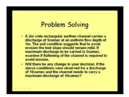
Will there be any change in your decision, if the above conditions were observed for a discharge of 10 cumec, if our discharge would have been 10 cumec, that means, say rather than 5 cumec for a 10 cumec of discharge, if we were getting 1 meter of depth uniform flow depth, and if the channel need to carry 10 cumec of discharge, then will my decision change or will our decision change.
