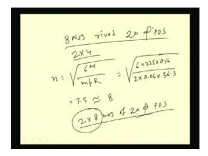
That means from load point of view, we can use eight numbers of rivet with 20 mm diameter power driven soft rivet. Eight numbers means if we use in two rows, then two rows with four numbers of rivet; means four numbers of rivet in each row we can provide, then we can make it. So, from load point of view we can find out this much number. Now let us see from the moment point of view. From moment point of view how do I find out the number?
