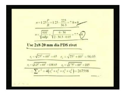
And accordingly, we can find out the total number of rivet required that is coming around eight from this. That means eight number of rivets is required from load point of view and from moment point of view it s required eight number of rivets with two rows.
