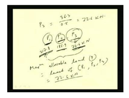
So, from this I can find out P 3 is equal to 36.3 by 0.5; that means 72.6 kiloNewton. So, for three types of joints, three allowable load we have derived P 1, P 2 and P 3. P 1 we have got from the connection between girder and angle; P 2 the permissible load due to the connection between angle and bracket, and P 3 is the permissible load due to connection between bracket and column. And in P 3, we are getting 72.6 kiloNewton.
