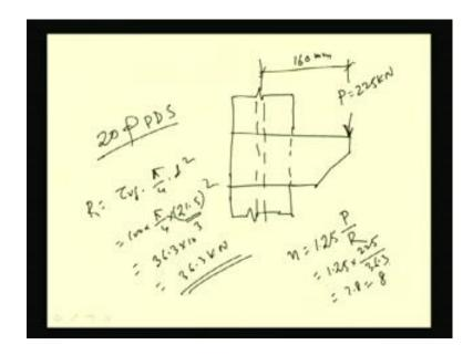
So, let us go through one example. Say, this is an example, say one bracketed connection has to be made which will pass the load to the column and the rivet joint has to made in such a way that without failure it can pass this much load. Say, P is equal to is given 225 kiloNewton. And the eccentricity is eccentricity is this one; this is say 160 mm eccentricity is given, right. Now with this we have to design the connections.
