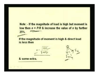
Now first, when we are going to design a riveted joint, we have to know what is the number of rivet? Now number of rivets can be decided in either from this equation that n is equal to P by R, where P is the load which is coming into picture, and R is the rivet value or from this equation that n is equal to root over 6 M by m R p, where M is the moment on that basis.
