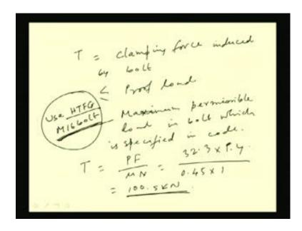
So, with all these we can find out the value of T. T means T is basically we can say clamping force induced by bolt which should be less than or equal to proof load. That means maximum permissible load, right. So, maximum permissible in bolt which is which is basically specified in the code, right. So, we can find out now the value. Say, T is equal to we are getting now P F by mu into N.
