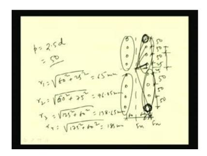
So, 16 rivets are placed in two rows. So, 8 rivets are placed in one row. So, let us place an let us find out the details of those. So, these are the pitch distance, say pitch distance can be found out from the caudal provision that is 2.5 d around we can make. So, this is becoming 50. So, let us say the pitch distance is 50, and this distance we have made 60, right. So, the neutral axis will be passing through this. So, this is 25; this will be 25, again 50, 50, 50.
