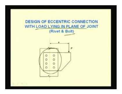
So, this difference will be there. So, the way we have designed in case of direct axial forces while coming into picture the bolt we have designed. So, in similar way we will design here also for the bolted connections. So, we will see those things. And our focus
