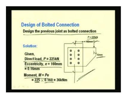
That means we will design another joint means same problem whichever we have done for riveted connections, we will design through the bolted connections. So, let us see that design the previous joint as bolted connection; previous joint means same values we will take. That is force is 225 kiloNewton with eccentricity. Eccentricity is 160 mm and 10 mm bracket has been used; we have to design the joint using the bolt, okay.
