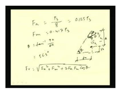
So, here F a will become P 3 by n is eight, total number of rivets have been given eight. So, this should become 0.125 P 3. So, one is vertically F a which is 0.125 P 3. Another is because of moment this at 90 degree angle to this radius, this is Fm and these value are F m we got 0.417 P 3. F m we got 0.417 P 3. So, F a we got and F m we got. Now we can find out the resultant. To find out the resultant, we have to know the angle.
