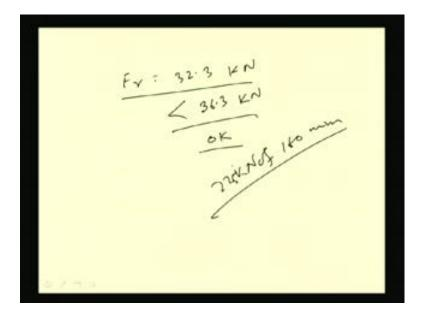
So, after calculating this value, we are getting F r as 32.3 kiloNewton. So, resultant force is coming 32.3 kiloNewton. This is the maximum force excreted on the rivet which is less than the rivet value. Rivet value is 36.3 kiloNewton for this particular diameter of rivet. So, this is okay; that means the joint is safe. That means the configuration whatever we have made; the number of rivets whatever we have assumed or we have calculated is safe to carry that much load.
