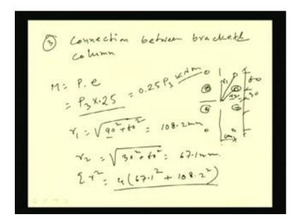
So, next will be the connection between bracket and column. So, third one will be connection between bracket and column, so connection between bracket and column if we see. So, what we will get?
