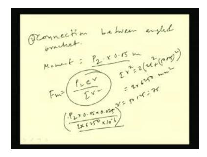
Another is the connection between angle and bracket. So, if we see the connection between angle and bracket, this two angles are connected to the bracket through four rivets and each rivets are in double shear because of two angles are located. And the eccentricity is 50 mm; the load is acting here, and we have to make connections here. So, 50 mm eccentricity is there. So, moment is there as well as the direct load is there.
