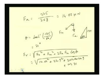
Another force is due to the direction load; that is direct load was applied 225 kiloNewton and total rivet is 2 into 8 means 16 rivets. So, this is coming 14.06 kiloNewton. So, one is this is F a, and this is F n, right. Now we have to find out the angle between these two; angle between these two you have to find out. Now, theta can be found out; from this if we see theta will be nothing but this one from which we can find out.
