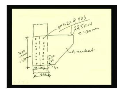
So, the design will be like this. This is the bracket. This load is here. Now this is the CG. So, in this way it has been one two three four five six seven, okay; so eight rivets in each group. So, this is, say h distance let us consider, say 40, and these are 50. And this is 120, then 60 into 60, and, say this is take as 40. So, we are assuming s distance as 40. So, this total depth of this will become 7 into 50 plus 2 into 40; that means 430, 430 mm is total distance.
