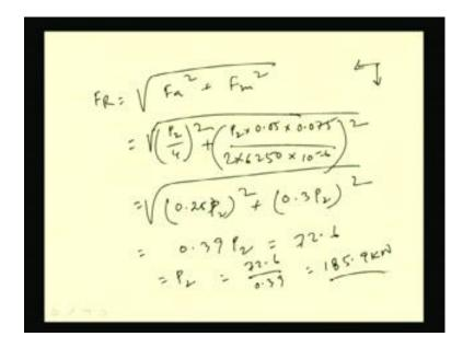
So, the resultant value F r will become F a square by plus F m square because both are acting perpendicular to each other. So, we can find out F a will be the four number of rivets, so P 2 by 4 if P 2 is the permissible load. So, this is F a and F m will be P 2 into 0.05 into 0.075 by 6250 into 10 to the minus 6, 2 into this. This is F m; this is F a. So, from this I could find out this is as 0.25 P 2 plus 0.3 P 2 whole square. So, finally, I am getting 0.39 P 2, right.
