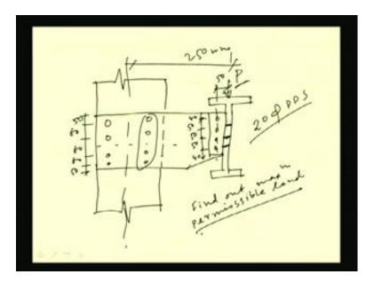
First if we see the diagram, there are four number of rivet in each row it is there. So, we have to find out if P 3 is the value, then we have to find out the resultant coming for a particular rivet. So, four number of rivets are there in each row. So, these distances are also given, okay. So, first we will find out M; M is equal to P into e. So, moment coming
