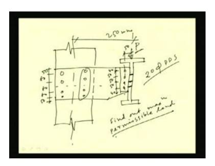
Now we will go through another example how to calculate and how to find out the allowable load of a particular joint. Joint is given in different ways; three type of rivets has been used. So, let us see through this picture we will able to understand. So, there are four rivets in each row. So, these are the rivets have been given. Again, say this is another plate and a gantry girder is carrying the load. This is P with an eccentricity of, say this is 250 mm. So, eccentricity is 250 mm.
