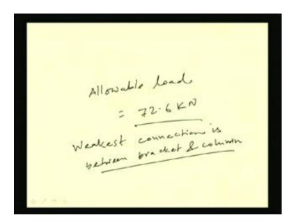
So, in the way we can find out the allowable load on this connection is coming 72.6 kiloNewton. And we can say the weakest connection is the joint between angle and bracket; weakest connection is between bracket and column, right. So, first failure will happen here, after that the second; that means the connection between angle and bracket.
