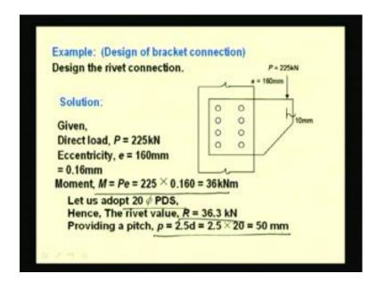
Now just let me overview that what I have done. First we have to find out the moment, what is the moment we have. Then the rivet value considering a particular diameter of rivet has been used. And accordingly the pitch has been decided as 2.5 d; that means 50 mm.
