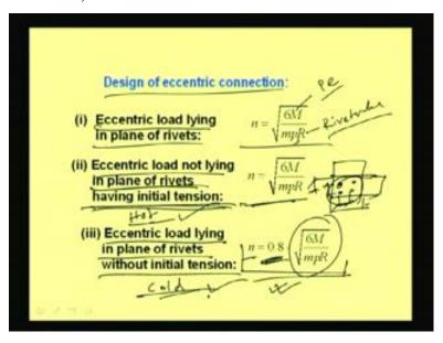
Now design that is design of eccentric connections how to design different type of connections? So, there are three type of things we have experienced. One is that eccentric load lying in plane of rivets. In that case, the number of rivets can be calculated as this n is equal to 6 M by m p R, where m is the moment due to eccentric load which is nothing but P into e, and R is the rivet value; that means one rivet which can carry.
