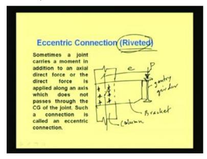
Today's lecture, we will be focused on the eccentric connection using riveted joints. When the forces are not acting through the CG of the joint, then the eccentricity will appear. So, because of that eccentricity additional moment will come into picture, and because of that moment, the rivet will exert some forces and that additional force has to be taken care properly. Let us see how it develops; say one column it has to pass the load from the beam, say from the gantry girder.
