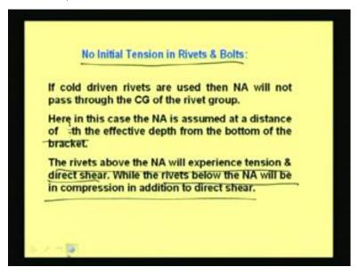
Now another case may happen which is called no initial tension in rivets and bolts. This happens when the cold rivets are used. In case of cold rivets, the neutral axis does not pass through the CG of the rivet group. The neutral axis is assumed in generally one-seventh of the effective depth from the bottom of the bracket. So, these are the assumptions we use to make, and then with that assumptions we use to find out what is the actual neutral axis depth.
