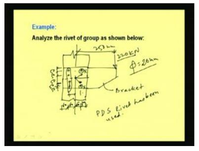
Now whatever I have discussed will be clear if I go through this example. Example is that to analyze a rivet group as shown below. So, let us draw the rivet group first, then we will see how we are going to find out the rivet value and how we will be checking whether the disjoint set is safe or not under this particular load. So, this is the, say column which has to carry the load through connections; say this is the bracket.
