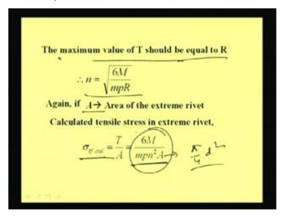
Now from this we can find out n. N is the number of rivet in one line. So, that can be find out as root over 6 M by n p R, right. So, using the maximum value as equal to the rivet value, we can find out n is equal to 6 M by m p R. Now again if we consider A as the area of the extreme rivet, then the tensile stress in extreme rivet will become T by A which will be 6 M by m p n square into A, right, where A is equal to pi by 4 into d
