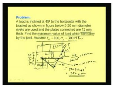
Another problem we will do through which we will be understanding how the load direction is going to change the calculation and how this direction of load is effecting on the rivet drop. Say the problem is given like this; say a load is inclined at 45 degree to the horizontal with the bracket as shown in figure below. Figure I am going to draw.
