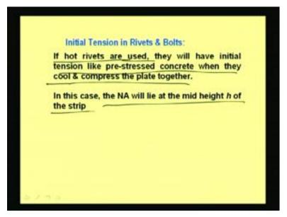
So, there are two type of case it can happen in case of rivet and bolts. One is the initial tension in rivets and bolts. Initial tension when it will come? When watt rivets are used. Power driven hot shaft rivets are used, then initial tension will come. Basically, they will have initial tensions like pre-stressed concrete when they cool and compress the plate together. So, in this case the neutral axis lie at the mid height of the strip.
