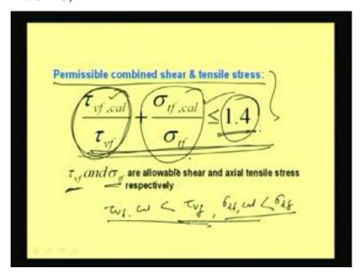
Now another thing is that permissible combined shear and tensile stress. So, if shear stress and tensile stress develop in the rivet, then we have to check that whether it is exceeding shear stress and whether it is exceeding tensile stress and jointly with this
