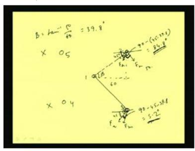
So, now to start with say let us make in a larger scale the rivet, so we will be able to understand. Say, this is one rivet, this is another rivet, rivet, rivet, and let us make it some numbering. Say, this is one, this is two, this is three, this is four, and this is five. Now, say first let us try to analyze this rivet. Now F a will be in this direction; that means with horizontal it is 45 degree angle, right.
