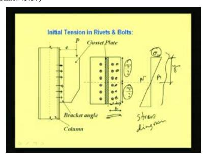
So, the stress diagram will become like this. This will be the stress diagram. This extreme fibers stress. So, this is sigma b t. So, stress will develop like this where this is the neutral axis at the middle and this is n p by 2; this is n p by 2. This can be called as b. So, due to the eccentricity, the stresses will be developing like this. This is the way which has been developed.
