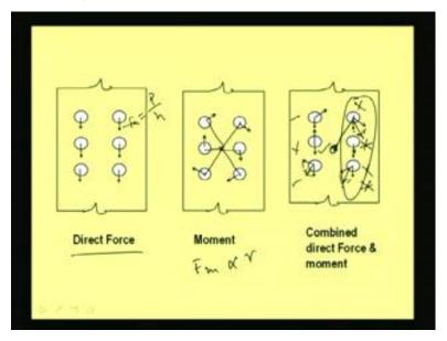
So, before going to M a let us see what I was telling the direct force always is coming F a. This is basically F a which is basically P by n; n is the number of rivets. In this case these numbers of rivets are six. And moment is developing like this if the center is here. So, it will be with 90 degree it will be like this; what I have shown earlier slides. And the combined force will be becoming like this.
