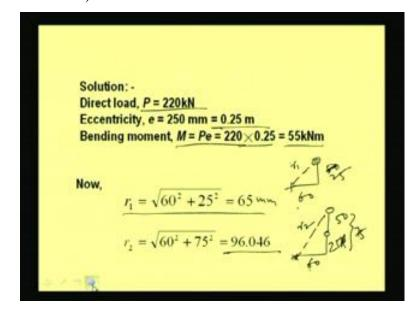
That is we know the direct load which has been given that is 220 kiloNewton, and eccentricity is given 250 millimeter or 0.25 meter. So, bending moment can be calculated as M is equal to P e is equal to 55 kiloNewton meter. Now summation r square we have to make. So, summation r square means first we have to find out the r. So, first r we will find out this one, this rivet.
