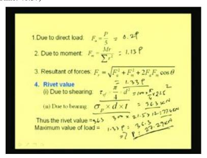
So, F a we are going to get 0.2 P, F m we are going to get 1.13 P and F r we are going to get the resultant force in terms of P as 1.33 P. Now due to shearing, the rivet value will become tau v f into pi by 4 into d square; that means 100 into pi by 4 into 21.5 square. So, this will become 36.3 kilometer. Similarly, due to bearing, this value will become 300 into 21.5 is the diameter, and thickness is 12 mm near to 77.4 kiloNewton.
