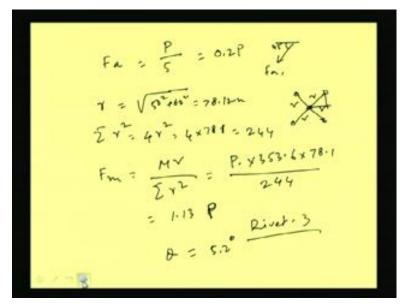
Say, F a we can find out as P by 5 because five numbers of rivets are there. So, this is basically 0.2 P. And this direction will be 45 degree to the angle. This is 45 degree, and this is F a, okay. And F m can be found out, okay. Before going to find out F m, let us find out r, r in the extreme rivet; means four corner rivets. That will become basically because this will be the r if rivets are there. So, this is r. This is the r. R will be basically this plus this square.
