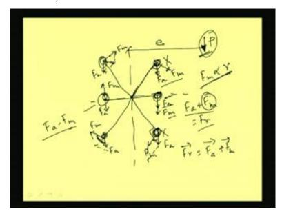
So, on a larger scale let us see how the forces are going to develop, say these are the some rivet group. So, six rivets are there let us assume, and let us assume that this is the center of the rivet group. Now the force p is acting here with an eccentricity e. So, this rivet will exert a force due to direct axial forces F a and due to eccentricity Fm due to moment, because of eccentricity of the load. So, this Fm will be basically acting 90 degree to this.
