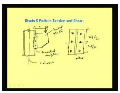
So, now we will be going to discuss about the rivets and bolts in tension and shear; that means tension as well as shear is going to be applied here. So, if the moment is not applied in the plane of rivet, in that case generally this happens. So, let us see how it looks like. So, if this is the column and this is the bracket and say this is the rivet which has been left, right.
