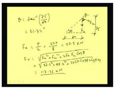
Now we have to see what is the angle between the F a and F m because F a is this one F m. So, we have see what is the angle this theta. So, that also we can find out because if I see this is the theta which will become this one. So, this theta can be found out; this is the distance which was given as 60, and this is the distance which was given as 75. So, theta can be found out from this which is coming 51.34 degree.
