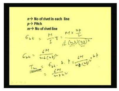
So, now if I consider the n as number of rivet and p as pitch and M as number of rivet line, then we can find out the value of sigma b t. So, sigma b t can be found out from this formula that M by I into y. So, M by I into y; that means M into y means basically from here to the extreme fiber distance this is y. So, this is basically n p by 2 and I is nothing but 1 by 12 m b into n p 1 by 12 b d cube. B means how many rows are there.
