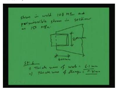
Stress in weld as 108 MPa and permissible stress in the section as, say 150 MPa. So, these are the data which has been given; now we have to design this. Design means we have to connect these members this channel sections though one gusset plate, so that the
