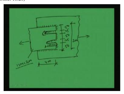
So, now if I draw the welding joint, it will look like this. Say, this is the channel. Now this is one slot weld we are providing. Then again another slot weld we are going to provide here, then like this. Now this is the gusset plate which has been joined. Now this is ISMC 200. So, if I go for welding, welding will be like this. So, remember that this portion will be circular means in a circular way we have to make it. So, welding will be in this way, right.
