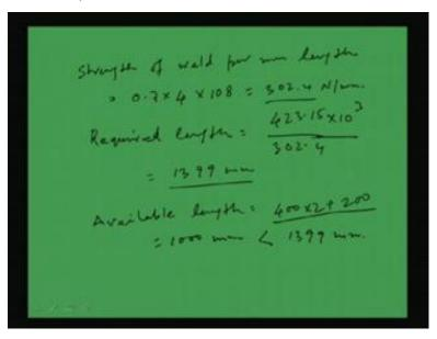
So, strength of weld per millimeter length can be found out. That will be now strength of weld how do we find out? Generally 0.7 into s is the throat thickness. So, 0.7 into the size of the weld is 4, and permissible stress in weld is considered as 108. So, this is coming 302.4 Newton per millimeter. So, we have to design the weld for the force of 423.15 KiloNewton.
