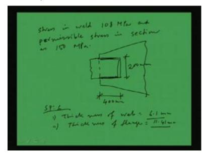
Because this is the available length; this length, this length, this is 400 into 2 plus this channel height. So, this length will be available which is coming 400 into 2 plus 200. This will become 1000 mm, right which is less than the required length 1399 mm. So, thus we need to provide an additional length of weld in terms of slot. So, what we will do?
