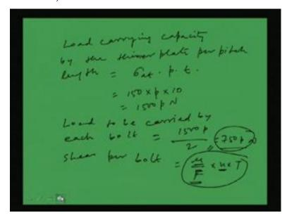
So, the load carrying capacity by the thinner plate per pitch length will be sigma AT into p into t. So, as in the question it is given that assume that permissible axial tension in plate as 150 MPa. So, I can find out the load carrying capacity as 150 into p into t is 10 mm thinner plate thickness. So, this is becoming 1500 p Newton. Now load to be carried by each bolt will be half of this because we have doubly bolted lap joint.
