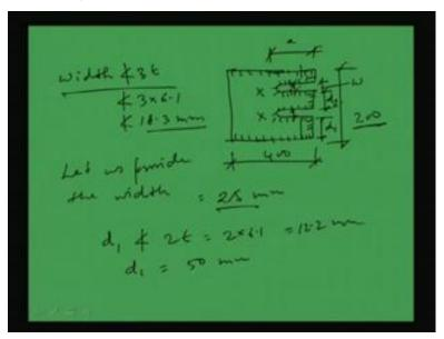
Say, let us assume this slot length as a. If this is the slot length, then I can find the value of a. So, how do I find out? So, this can be found out, say a will become 1399 minus 1000 by 4 a because. So, this length if it is a; so, a plus a plus a plus a; that means this 4 a. So, 4 a will be equal to the rest length that is 399. So, 399 by 4 that will become 100 mm; so, the length of the slot will become 100 mm. So, in this way I can find out.
