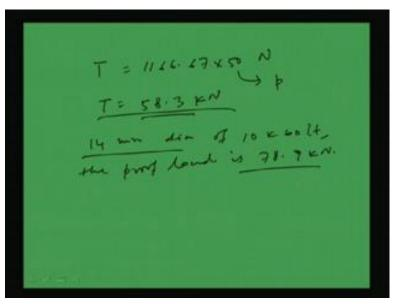
So, from this calculation we can find out t as 1166.67 into 50 Newton assuming the pitch as 50 mm. Means the same problem we are doing considering all other things same, except the plate thickness we are making same that is 10 mm, and the number of interface in case of butt joint will become 2. So, t is becoming from this as 58.3 KiloNewton. So, t is becoming this.
