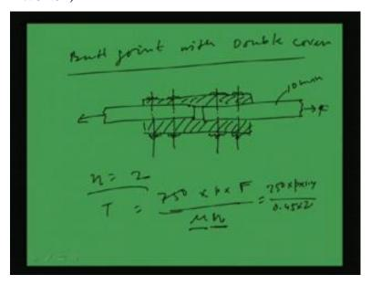
Now let us design the same plate considering butt joint with double cover, right. Now in case of butt joint, what will happen? So, it will look like this. Let us assume the plate thickness of two plate is same, right. Say, one cover is given here, another cover is given
