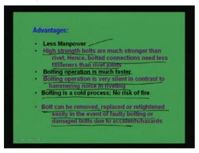
Now let us come to advantage and disadvantages of bolting. Now what are the advantages? The major advantage in bolt connection is one that is less manpower. Because manpower will be very less, because if you have the bolt along with the nut, then one can tighten the plates at this side very quickly, and there will be no requirement of other things like heating or like some hammering; nothing will be required, just you can tighten.
