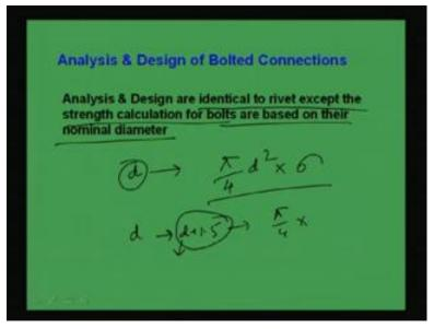
Now let us go to the analysis and design of bolted connections. So, as we told that analysis and design are identical to rivet except the strength calculation for bolts which are based on their nominal diameter. In case of bolt, we know the nominal diameter; what are the nominal diameter of the bolt? So, from that we can find out the strength, because the stress we know permissible stress in a particular bolt with a particular type of material. We know what is the permissible stress?
