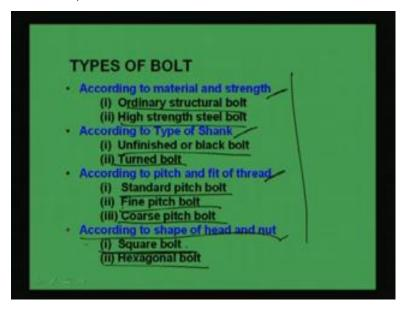
Another way of classification is according to the shape of thread and nut; that also can be classified which is called square bolt and hexagonal bolt. So, what we are seeing here that types of bolt can be categorized as per their different parameter like according to material and strength according to shank type, according to the pitch and fit of thread,
