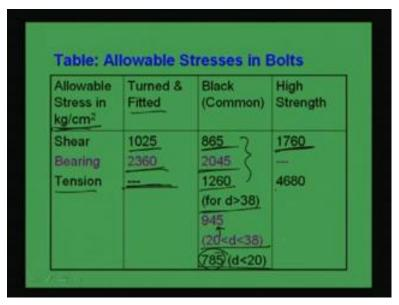
And earlier we have discussed we have shown what are the stresses for different type of rivets which are given in the code. Here I am showing in the table that what are the allowable stresses for different type of bolt and for different type of stress; like for turned and fitted bolt, the shear stress is 1025, and permissible shear stress for black common type bolt is 865. This is in kg per centimeter square. And for high strength bolt, the shear stress will be 1760 kg per centimeter square.
