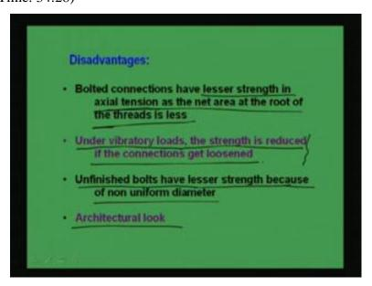
Another is which is very, very important that is under vibratory loads, the strength is reduced if the connections get loosened because of vibration the strength may reduce, because of vibration it will go to loosen the connection. So, for that the strength will be
