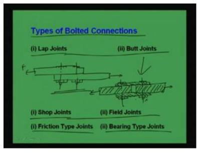
Earlier we have decided type of bolt. Now let us discuss about type of bolted connections. Now what is the type of connections through bolting we used to use. So, one is that we can connect as a lap joint or as a butt joint. This is one important connections, which through bolting we used to do. How it looks like in case of lap joint or butt joint let us see. In case of lap joint say two plates are left and, say force is acting like this.
