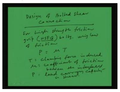
Now, say let us discuss about the design of bolted shear connection, how to find out the stress of the bolt and how to design it. Now for high strengths friction grip bolt, now onwards we will tell that HSFG high strength friction grip bolt using law of friction, we can write P is equal to mu into T. So, using law of friction, one can write P is equal to mu into T for high strength friction bolt, where T is the clamping force induced.
