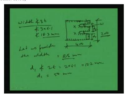
Now we have to find out the slot length and its distribution. That means slot length means we know that we are cutting though the plate up to some length and then we are distributing accordingly. Say, let us make like this, say this is the total over length length. So, this is 200 and, say this is 400. So, extra length we are providing through making
