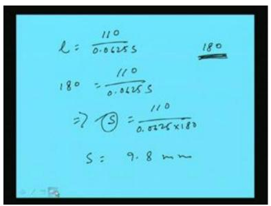
So, the required length will be becoming 110 Kilo Newton was there. So, 110 by 0.0625 S, okay and here we have seen the maximum length of the weld was 180. So, maximum we can provide 180, right. So, 180 will be equal to 110 by 0.0625 into S. So, from this I can find out the value of S which is becoming 110 by 0.0625 into 180, because 180 is the maximum length which we can provide. So, length is fixed; we can find out the value of S, right. So, from this we can find out S as 9.8 mm.
