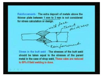
Now another parameter is called reinforcement. Basically, the extra deposit of metals above the thinner plate between one millimeter to three millimeter is not considered for stress calculation or design. So, this is basically called extra deposit basically. Now if we see in the picture how it looks like let us see; say, one plate is given like this which has to be welded by the butt, and the plate is this which is like this.
