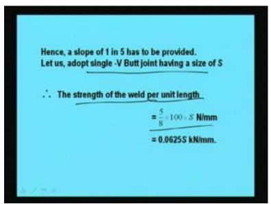
So, that means using single-V butt joint we are going to get the strength of the weld per unit length as this 5 by 8 into 100 into S which is coming 0.0625 S Kilo Newton per meter.
