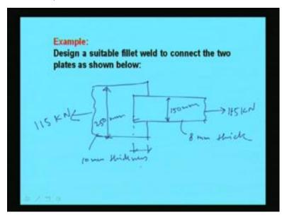
Suppose, we are considering this example; the design is suitable fillet weld to connect the two plates as shown below; say, suppose one plate is connected like this, and another plate is overlapped like this. Now so overlapping length is basically this much. Now this is having 115 Kilo Newton tensile force in this plate. So, we have to joint these two plate with the fillet weld.
