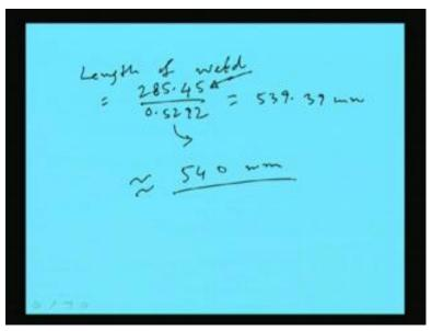
So, length of the weld will become 285.45 by 0.5292. This is the strength of weld per millimeter length, and this is the strength of the plate which can be carried by the angle. So, this is coming 539.39 millimeter; that means we can use 540 millimeter. So, 540
