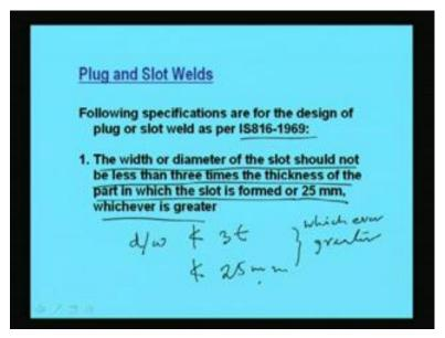
Now some specification has been given by IS816-1969. So, I will discuss some specification on the basis of which we have to design the slot weld or plug weld. So, before designing the slot weld and plug weld, we have to know what are the restriction given by the code. And according to that what will be the specification of the slot weld? What will be the distance d? What will be width? What will be the diameter of the slot? All these things will be given here.
