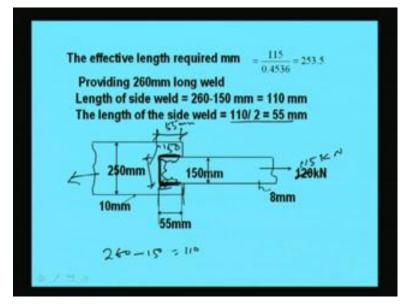
So, if we design it will look like this, say, the plate is there. So, we can provide, say, this length is becoming 150. So, 150 means we have provided 260 mm length; so 260 minus 150 that is 110. So, 110 millimeter length has to provide in this and in this area. So, that means 110 by 2 which is becoming 55 mm. So, the length of the side weld will be 110 by 2 is equal to 55 mm.
