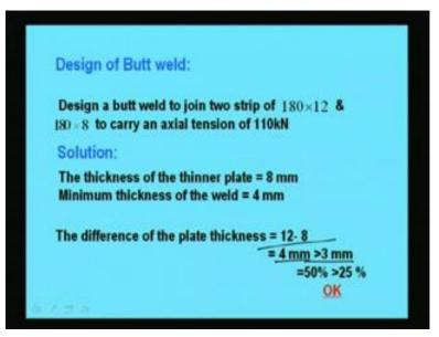
So, the difference is becoming 4 mm which is greater than 3 mm, okay. What we have seen from the codal provision as that difference will be how much. This is 50 percent; that means this is greater than 25 percent. So, it is okay. So, accordingly we have to make it, right.
