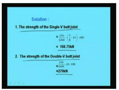
So, in this way we can find out the strength of the single-V butt joint as 168.75 Kilo Newton. And strength of the double-V butt joint can be calculated as 270 Kilo Newton.
