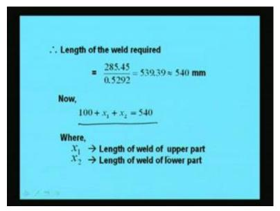
So, what I was discussing that 100 plus x 1 plus x 2 will become 540, where x 1 and x 2 has the length of upper part and lower part of the plate, where x 1 is the length of weld of upper part, and x 2 is the length of weld of lower part.
