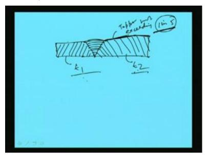
Say, one plate is something like this. Now this can be joined like this. So, this is the welding place, and this tapering will be not exceeding one in five. So, this tapering should not exceed one in five in this ratio. So, this is how the joint look like, say this is one plate and another plate is this; that means this is the plate. Now we are tapering in this way, then the butt weld is given here.
