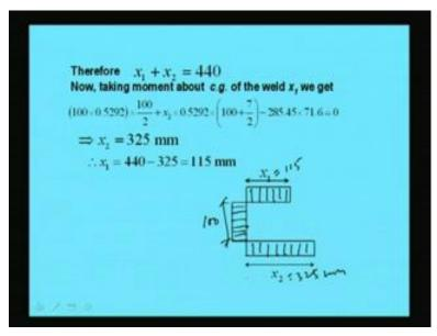
So, that is what we have calculated. So, x 1 we are going to get 115 which is welded here, and x 2 we are going to find as 325 mm which is in this side, and this is along its height. This is 100 mm which was fixed due to its dimension of the angle. So, in this way we can find out the welding length as well as the distribution of length in around the plate. So, in this way we have to design. So, I hope like this type of problem.
