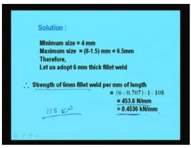
That means the strength is becoming this much 435.6 Newton per millimeter or 0.4536 Kilo Newton per millimeter. That means strength of the weld we are calculating per millimeter length as 0.4536 Kilo Newton. Now applied force is 115 Kilo Newton. So, the length we can find out from this formula.
