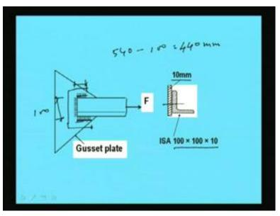
So, we can see the figure that we have a gusset plate. This angle has to be joined with this which is thickness of 10 mm. The angle size is 100 by 100 by 10, and it has to take the maximum load and the fillet weld has to be made in this way; means in this periphery the fillet weld will be. So, like in earlier case the minimum size we know.
