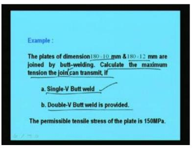
The two plates of dimension 180 by 10 and 180 by 12 mm are to be joined by the butt weld. Now we have to calculate the maximum tension of the joint; for tension the joint can carry using single-V butt weld and double-V butt weld. So, if we provide single-V butt weld, what will be the maximum tension it can carry by the joint, and if we provide double-V butt joint, what will be the tension it can carry, assuming the permissible tensile stress of the plate as 150 Mpa.
