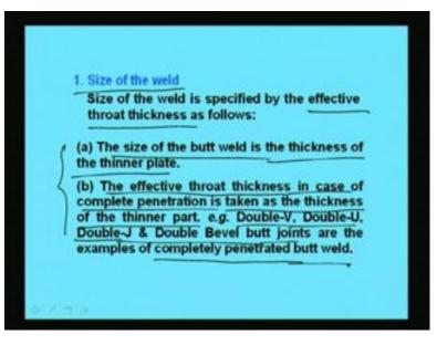
So, when we are seeing this size of the weld, so how to find out the size of the weld? So, as per the codal provision, the size of the weld is specified by the effective throat thickness which is given below, effective throat thickness how to find it? The size of butt weld is the thickness of the thinner plate; that means the size of the butt weld can be assumed as the thickness of the thinner plate where we are going to joint; this is one.
