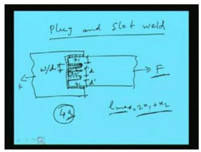
Now another type of joint we used to do which is called plug and slot weld; what is this? That we know, say, one plate is like this and, say, another plate is like this which has to be joined with some load. Now if force is becoming more, then length of the weld will become more. Length of the weld will become more. But we cannot go beyond a certain length because this length is fixed. Maximum length will be, say, this is x 1, and this is x 2.
