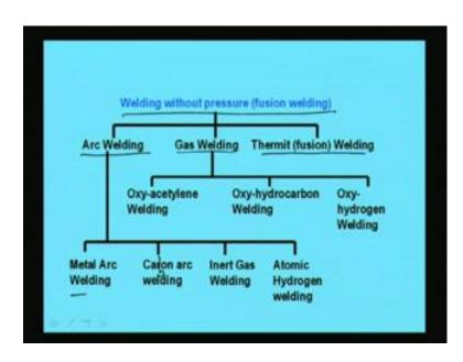
Then this welding without pressure this can be classified into 3 categories. One is called arc welding then gas welding and another is thermit or fusion welding. This arc welding can be of metal arc welding, carbon arc welding this will be carbon arc welding, inert gas welding and atomic hydrogen welding. And gas welding will be oxy acetylene welding oxy hydrocarbon welding and oxy hydrogen welding. So, these are the different categories of welding.
