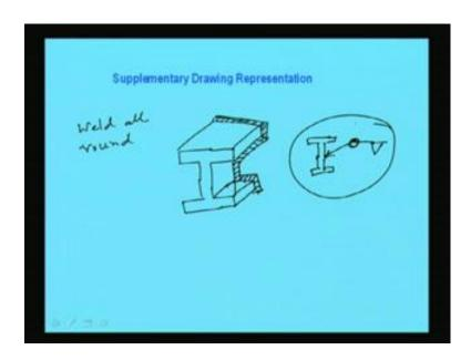
Another one is weld all round the form of weld is weld all round. If it is like that then the section will be like this. So, suppose one I section is given now, if I see in the 2 dimensional it will look like this and this will be forming in this way. These are basically forming by weld all around this will be, so this will be like this. So, that basically forming all around, so drawing representation will be simply like this just you give the I section then is it given like this.
