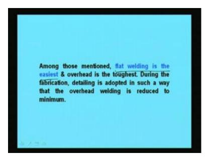
Now, among those mentioned these 4 types of welding. Flat welding is the easiest and overhead is the toughest. During the fabrication detailing is adapted in such a way that the overhead welding is reduced to minimum.
