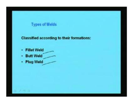
Now, types of weld, basically these are divided into 3 types on the basis of the formation. How it is forming? This is one is called fillet weld another is butt weld and then plug weld. So, this basically this 3 type of weld will be looking for designing of steel members. So, we will see all these in details later.
