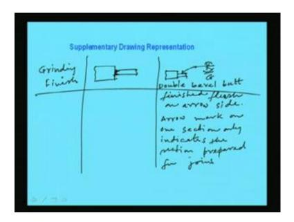
So, in this way we can represent few more welding types which is the form of weld will be grinding finish. Grinding finish and the section will be looking like this and the drawing representation will be like this. This is grinding finish this will be like this and this is basically double bevel butt finished flush on arrow side. Here arrow mark on 1 section only indicates the section prepared for joints prepared for joints. So, in this way the drawing representation will be there.
