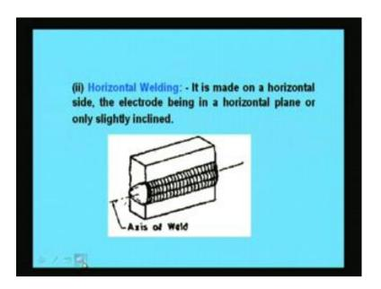
Next in case of horizontal welding it is made on a horizontal side the electrode being in a horizontal plane or only slightly inclined. Axis of weld will be in this way and welding will be in this cases.
