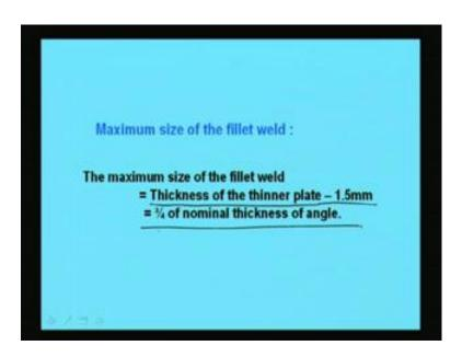
Now, maximum size of fillet weld that has been guided by the code as the maximum size of fillet will be the thickness of the thinner plate minus 1.5 mm this will be the maximum size of the fillet weld. Thickness of the thinner plate minus 1.5 mm and this will be three-forth of nominal thickness of angel. If it is connected by the angle then this will be three-forth of nominal thickness of the angle.
