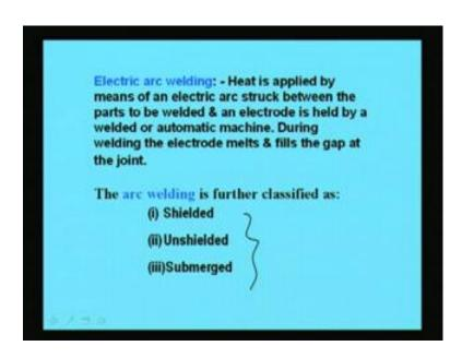
The mostly used welding is electric arc welding where heat is applied by means of an electric arc stuck between the parts to be welded and an electrode is held by a welded or automatic machine. During welding the electrode melts and fills the gap at the joint. The arc welding is further classified into these 3 category; one is called shielded another is called unshielded and then submerged.
