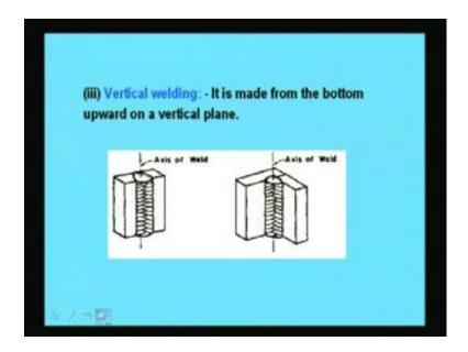
Another is vertical welding it is made from the bottom upward on a vertical plane. Axis of weld will be vertical and the 2 connections 2 members can be connected in this way which is called vertical welding.
