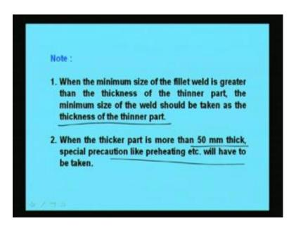
Now, you have to note the following points. One is the when the minimum size of the fillet weld is greater than the thickness of the thinner part. The minimum size of the weld should be taken as the thickness of the thinner part. So, you have to remember this point. Another point is when the thickness part is more than 50 mm thick special precaution like preheating etcetera will have to be taken care properly. So, this is another important part while joining the 2 plates with welding.
