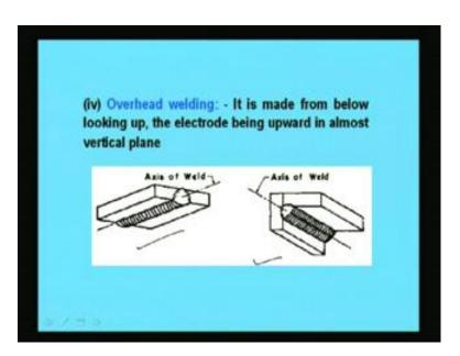
Next is overhead welding. It is made from below looking up the electrode being upward in most in almost vertical plane. This is looking like this axis of weld will be like this or like this and it is connecting in this way.
