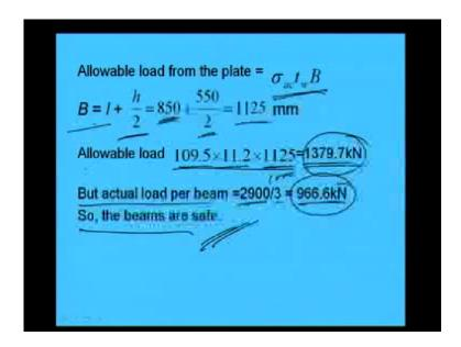
Now, allowable load from the plate will become sigma a c into t w into B, sigma a c in to tw into B. Now B will become how much L plus h by 2, L was 850 and h was 550. So, 850 plus 550 by 2 which is becoming 1125, 1125 millimeter. So, B is becoming 1125 millimeter. So, allowable load we can now find out that is 109.5 into 11.2 into 1125. So, this is becoming 1379.7 kilo Newton. So, allowable load we are going to get 109.5 into 11.2 as t w into b is 1125.
