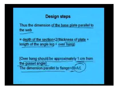
Then the dimension of the base plate parallel to the web can be calculate from this that is depth of the section plus 2 into thickness of plate plus length of the angle plus over hang. Over hang should be approximately 1 centimeter from the gusset angle and the dimension of parallel to flange B will become A by L, A is the total means area.
