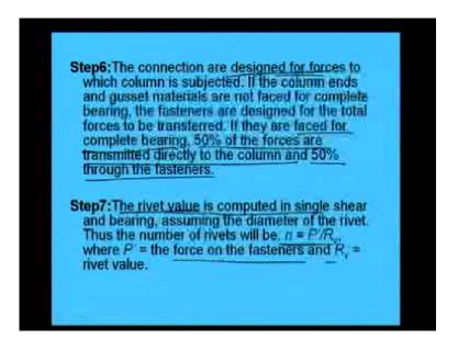
Then the connections are designed, then the and this connection are designed in decision of that 50% of the forces will be transmitted directly to the column and 50% through the fasteners, if they are faced for complete bearing otherwise whole. And we can find out the rivet value for a particular diameter of the rivet and blood thickness there you can find out the number of rivet. On the basis of force on the fasteners and rivet value.
