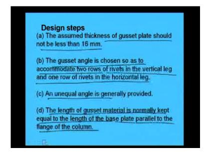
According to the some (())that like the assume thickness of gusset plate should not be less than 16 m m, this is 1. The gusset angle is chosen. So, as to accommodate 2 rows of
