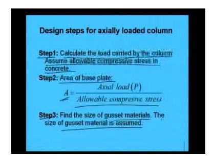
Just I am re writer it is (()) that is first step what will you do that calculate the load carried by the column and will assume allowable compressive stress in concrete specification, then area base plate will be find out that is axial load by allowable compressive stress in step 2. Step 3 will find out the size of gusset materials and that will be assumed.
