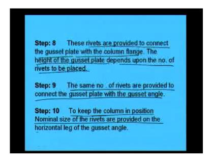
So, this are the state and rivets will be provided to connect the gusset plate with the column flange, the height of the gusset plate depends upon the number of rivets, the same number of rivets are provided to connect the gusset plate with the gusset angle and took column to keep the column in position, nominal size of the rivets are provided on the horizontal gusset plate.
