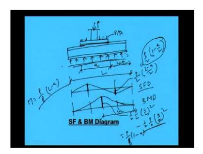
Now, before going to analyze let me show the shear force diagram and (()) diagram of the means footing how it is coming. Say, as you know suppose load is coming shift e then it this is resting on the base plate, then what will happen and then it is going say (()) the beam. So, well we are going to design this beam you have to know how much load is coming on this beam and how it is means where the maximum bending moment and
