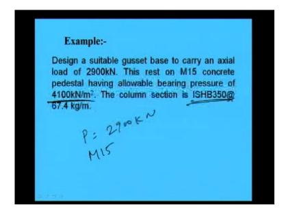
These are the thing and we have seen the example that load was 2900 kilo Newton and M15 grade of concrete was used bearing pressure of 4100 kilo Newton kilometer square and I S H B 350 where used. So, let us see.
