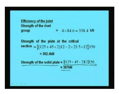
Again the strength of the solid plate will become means if rivet is not there if hole is not there then the strength of the solid plate will become this 1 125 plus 45 into 2 into 12 into 150. So, this will become 387 Kilonewton, now we have to find out the efficiency, so efficiency how do we find out efficiency will be the strength of the riveted plate by the strength of the solid plate.
