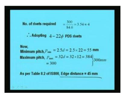
So, pitch distance we can find out now as for the table 8.2 of IS 800 the edge distance will become 45. So, with this we can find out the gauge distance and others dimensions.
