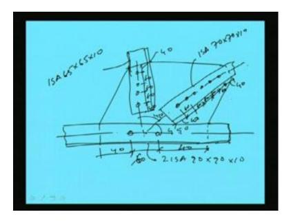
Say this is the button chord with having 2 angle this is 2 ISA 90 into 90 into ((01:01:20)) 10 this is the center line this is the vertical line. Now, another member is here another member is here another member is this 1, so this is 45 degree this is also 45 degree. So, we are providing some rivets if we are it is 4 number rivets will be required and the pitch
