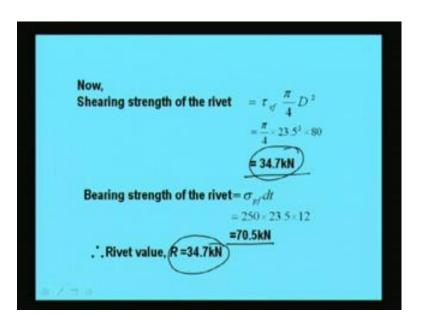
That means the shearing strength of the rivet we are going to get 34.7 Kilonewton and bearing strength of the rivet we are going to 70.5 Kilonewton. That means the failure will first accour, because of shearing strength, so we will find out the rivet as the lesser value of these 2; that means, 34.7 Kilonewton.
