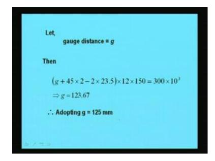
So, the process what we have discuss that how to find out the gauge distance and how to find out the total width of the plate. So, in this case we are adapting gauge distance as 125.
