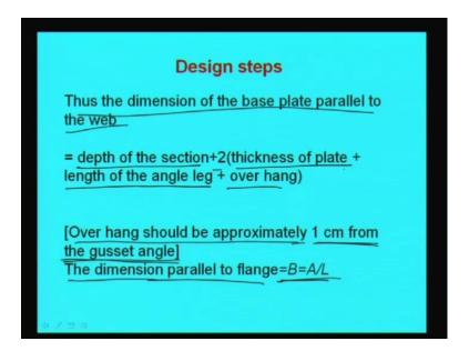
Thus the dimension of the base plate parallel to the web will become how much? That is the depth of section plus 2 into thickness of plate plus length of angle leg over hang. So, in this way, we can find out the dimension of base plate parallel to the web. Dimension of the base plate means; length or width of the base plate parallel to the flange of the column.
