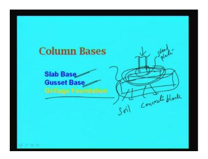
Three type of column base generally we used; one is slab base, which is called where load is little less. And then gusset base, where load is high and generally when the moment is also coming into picture eccentricity is coming into picture. And then another is grillage foundation. This generally nowadays we do not use, but still I will give a overview of grillage foundation also. So, this last module; will consist of 2 lectures and in 2 lectures I will try to cover these aspects.
