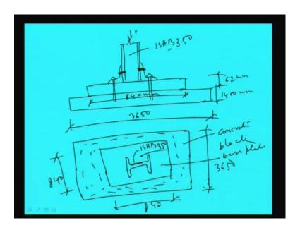
That if we draw the final outcome, we will see this is a. So, this is base plate right, then this is I am not going later, I will come means how to make connections right. So, here it is P was there this is ISHB 350. So, this is becoming how much 62 millimeter and this is 1400, 62 millimeter. This is not in scale 1400 millimeter right. And this will be the 3650 meter concrete length and width and base plate length and width will become 840 millimeter right.
