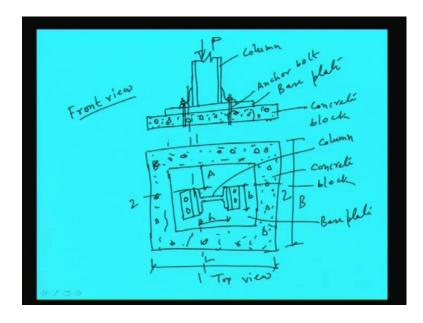
If we see w, if w is the uniformly distributed load, then w into A is this A square by 2. This will be the maximum bending moment here. Similarly bending moment in this
