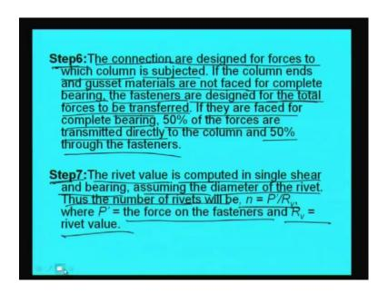
Now, in step 6 what we will do. In step 6, the connection are designed for forces to which, column is subjected. Connections are designed for forces to which column is subjected. If the column ends and gusset materials are not faced for complete bearing, the fasteners are designed for the total forces to be transferred. If they are faced for complete bearing, then 50 percent of the forces are transmitted directly to the column and 50 percent through the fasteners.
