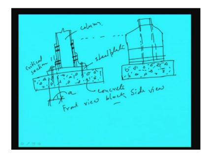
Let us see how it looks like. Say this is a column right and this will be the base plate, then concrete block right. Here we use to provide additional gusset plate here, to take care of the moment right. Now, this is front view and this the concrete block right. And critical sections will lie, where this will be in this. So, section 1 1 this will be the critical section through, which we have to design right.
