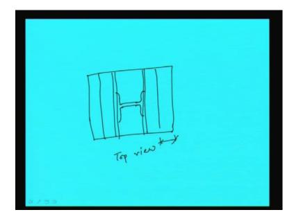
That we have shown in the picture if you remember you see, this one the length will be same with the gusset plate length right. So, the length of gusset material is normally kept equal to the length of the base plate parallel to the flange of the column.
