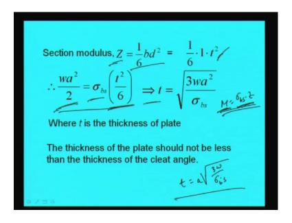
Again in the earlier case if we remember, in the same we will do. That section modulus z is can be written as 1 by 6 bd square and for a unit thickness, we can take 1 by 6 1 into t square right, where t is the thickness. So, the moment will become M is equal to sigma bs into z, where z is t square by 6. M is equal to sigma bs into z, moment carrying capacity is sigma bs into t and developed moment is M that is wa square by 2.
