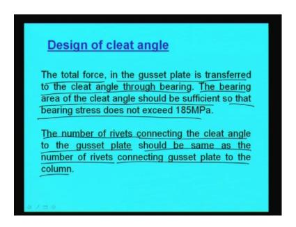
Now, another thing is cleat angle. We have to design the cleat angle. Now how do we design? That is the total force in the gusset plate is transferred to the cleat angle through bearing. We know total force is transferring to the gusset plate through bearing. So, the bearing area of the cleat angle should be sufficient so that, bearing stress does not exceed that specified stress that is 185 Mpa.
