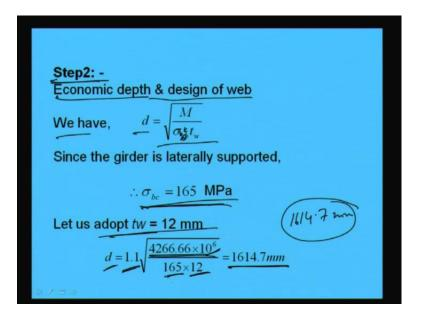
Next we will go to step 2, where we have to find out the economic depth and web means design of web. So, we will find out now, economic depth of web and accordingly we will design right. So, economic depth as we know will become M by sigma cb or bt into tw sigma bc or bt right into tw. Here sigma bc or sigma bt is 165 as it is laterally supported right.
