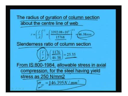
So, then what we will do. Now, we will find out the radius of gyration of column section about the centre line. So, radius will be I by A square root of I by A. So, I was found 3392.08 into 10 to the 4 and A is 15768. So, r will become 46.38 millimeter. And the slenderness ratio of column section will become I by r equal to 1776 by 46.38. That will become 25.365.
