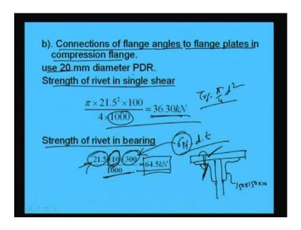
Now, we will go for connections. Now, connections of flange angles to flange plates in compression flange. Let us see how to connect flange angles to flange plates in compression flange. So, in this case also let us use 20 mm diameter of power driven rivets. So, strength of rivet in single shear will become pi by 4 into d square into tau vf tau vf into pi by 4 into d square, because this will be in single shear right. And 1000 has been divided because to make it kilo Newton.
