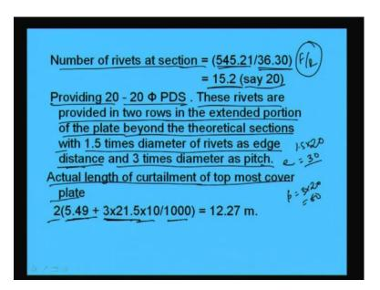
So, the moment we get rivet value we can find out the number of rivets at the section. So, what will be the number of rivets at this section? That will become the force whatever we got here right, the shear force 545.21 kilo Newton tensile force at the cover we found that by rivet value means F by R. Say from this we are going to get 15.2 right. So, we are going to get 15.2. And say let us use little high say 20 or 60 means 60 means minimum required right.
