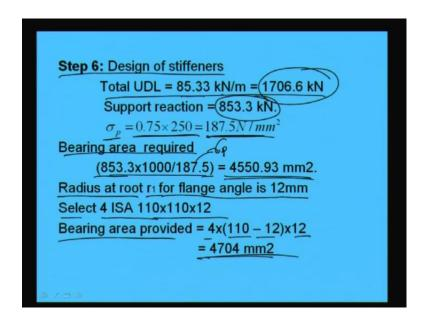
Next we will go for design of stiffener. This is the last step. So, as we know UDL load we have already including self weight, that is, 85.33 kilo Newton per meter. Then total load will become this. And support reaction as we have calculated as earlier. So, sigma p will become 0.75 into fy that is this. So, bearing area can be found from this equation that is 853.3 into 1000 by 187.5, because this is the sigma p right.
