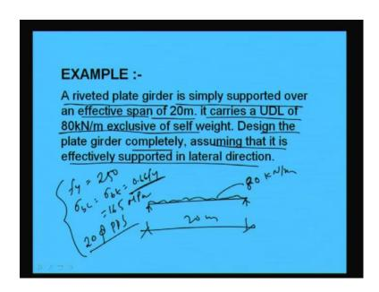
That is a riveted plate girder is simply supported over an effective span of 20 meter. So, span was 20 meter and it carries a UDL of 80 kilo Newton meter 80 kilo Newton per meter exclusive of self weight. So, this is 80 kilo Newton per meter, which exclude self weight. Design the plate girder completely assuming that, it is effectively supported in lateral direction, effectively supported in lateral direction. That means if let us consider fy is equal to 250.
