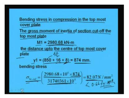
So, bending stress in compression in the top most cover plate can be find out and can be checked. Now, the gross moment of inertia of section cut-off, the top most plate M 1 will become this 1 right. And the distance up to the center of the top most cover plate y 1 will become this 850 plus 16. This is because dw by 2, that is, 1700 by 2 850 plus 16 plus 16 by 2. So, this is 874.
