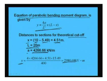
Value of bending moment we can find out from here right. As we know equation of parabolic bending moment diagram can be given here. y is equal to 4 a by L square into x into L minus x. Now, distances of 2 section for theoretical cut-off x can be found, that is, L by 2 this is 10 minus 5.49. That will be 4.51 and L is given this and area is given this. So, using this value we can find out. That is 4 into 4266.66 into 4.51 into 15.49 by 400. That will be this much; 2980.86.
