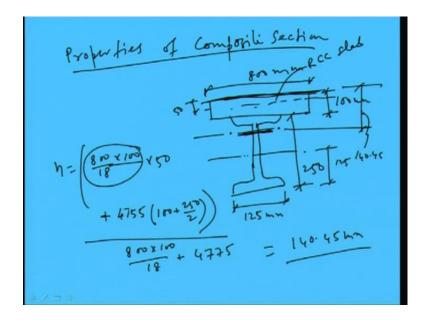
So, now we have to find out the properties of composite section. So, how do we find out? Say, property can be find out, let us draw the figure. Say, this is the effective width which is 800 millimeter, we find out. This is concrete slab, RCC slab. Then, the beam is given; this is the steel beam. Now, this width is 125 millimeter. And other things are like this is given as 250 because ISMB, 250 we have used; and the slab thickness is given 100 millimeter. So, these are the properties we know.
