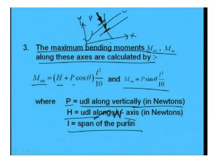
Now, next step is the maximum bending moments; the maximum bending moments M u u and M v v along this axis are calculated. What I have shown there that M u u will be equal to H plus P cos theta into l square by 10, and M v v will become P sin theta into l square by 10, where H is the, if purlin is provided here like this, so this is I section. We are considering H normal to this direction; we are assuming that wind force is coming normal to the purlin; So, H will be this one.
