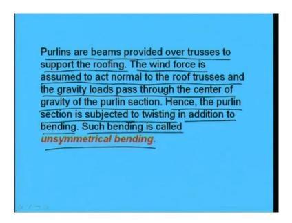
So, what I was telling, that purlins are beams provided over trusses to support the roofing. The wind force is assumed to act normal to the roof trusses and the gravity load pass through the center of gravity of the purlin section. Hence, the purlin section is subjected to twisting in addition to bending. Such bending is called unsymmetrical bending. So, chances means the unsymmetrical bending cases will happen, so I have to find out accordingly the stresses.
