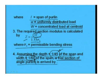
W is the concentrated load at centroid, and this w is the uniformly distributed load, and l is the span of purlin. So, in this way we can calculate the value of maximum bending moment. The moment we calculate the maximum bending moment we can find out the required section modulus.
