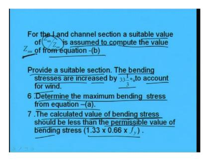
So, next what we will do? So, what I was telling that you see for the I and channel section a suitable value of Z u u by Z v v is assumed to compute the value of Z u u from equation b; equation b means this one. To find out a suitable section for channel and I say I, sorry, for channel and I section we can assume some ratio of Z u u by Z v v, then we can find out the value of Z u u.
