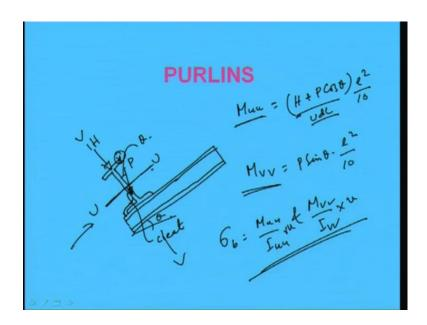
Now, I will discuss about design aspects of purlin. Purlin, as we know, when the industrial sets are designed, the wind force coming into picture at a particular direction, from a particular direction it used to come. So, when we will be designing a purlin, what we will see? Purlin is basically a type of beam. We will see, it is a, means it is having 2 type of load - one is gravity load which is acting vertically, another is wind load which is coming from horizontally.
