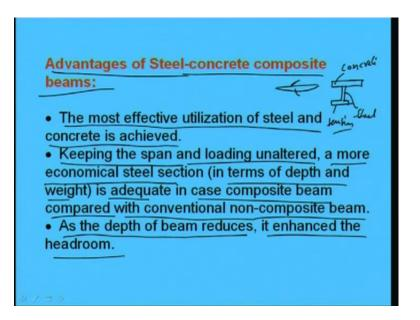
Now, let us see, what are the advantages of steel concrete composite beams? I have just written down here, just you can note that; one is the most effective utilization of steel and concrete is achieved, because if suppose there is a beam which is deflecting like this, then at the top the compression will develop and at the bottom tension will develop.
