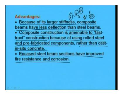
Another advantage is because of its larger stiffness, composite beams have less deflection than steel beams. So, as we know, the deflection depends of F is equal to k into d, where k is the stiffness, d is the displacement or deflection, F is a force. Now, if k is high, then definitely d will be less, because d is equal to F by k.
