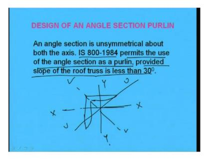
Now, similarly, we will discuss about the design of an angle section for using as a purlin. In angle section, it is an unsymmetrical section, so in both the directions the moment has to be calculated. In IS 800- 1984, it permits the use of angle section as a purlin, provided slope of the roof truss is less than 30 degree. So, if slope of the roof truss is less than 30 degree then IS means, IS code has permitted to use angle section also.
