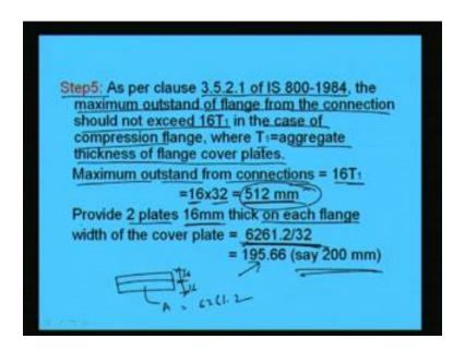
Now, let us come to step 5. As we know as per clause 35020.1 of IS 8984 the maximum outstand of flange for the connection should not exceed 16 T 1 in the case of compression flange where T 1 is equal to aggregate thickness of flange cover plates. So, maximum outstand from connection will be 16 T 1. So, 16 into T 1 T 1 is 32. So, we are going to get 512 millimeter right. Now, if we provide 2 plates of 16 mm thickness on each flange then width of cover plate can be found.
