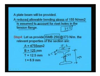
So, that is what I have written here a reduced allowable bending stress of 155 Newton per millimeters is assumed to account for rivet holes in the tension flange. Now, as the restriction is given that maximum height will become 350. So, we cannot go up to a
