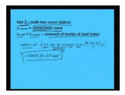
Now, we have to find out the net Zxx Zxx 2 with 2 cover plate right. As we know gross moment of inertia is this which has been calculated earlier 345952600 millimeter to the 4. So, net will be gross minus moment of inertia of rivet holes right. So, net let us find out. So, gross minus moment of inertia of rivet hole rivet hole is given here that is diameter into depth, depth means 2 plates were there. So, 18 plus 18 plus thickness of flange right d plus d plus tf this is the thing.
