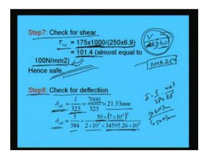
Now, what we will do. We will go to next step for checking of shear. So, for checking of shear as we know we have to find out the stress that is we know 175 kilo Newton it was. So, V is 175 kilo Newton which we have calculated. And this is the depth D and this is the web thickness tw means V by D into t sorry D into tw web thickness. So, from this we are going to get 101.4 Newton per millimeter square. And the allowable stress is tau here is 100 Newton per millimeter square.
