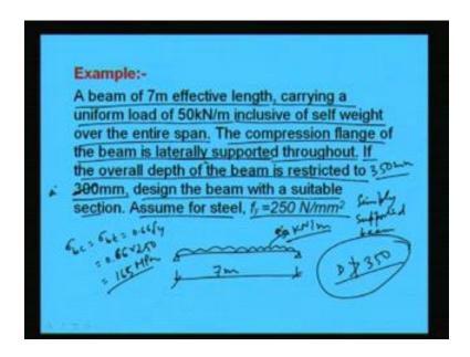
This example is like this that a beam of 7 meter effective length carrying a uniform load of 50 kilo Newton per meter including of self weight over the entire span right. The compression flange of the beam is laterally supported throughout. If the overall depth of the beam is restricted to 3 100 mm design the beam with a suitable section. Assume for steel fy has 2 50 millimeter right.
