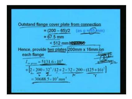
So, if you see earlier the gross area we have calculated like this you see this plus 2 into this plus this. This was 30688 into 10 to power 4. And here it is coming 34595 into 10 to power 4. So, it is going to increase. So, what we are doing for gross area that a moment of inertia of the section ISMB then moment of inertia about its own axis. That is 2 into b sorry b will be 200 bd cube by 12 plus A this is Ar square, right.
